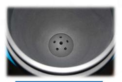
Coater converging section and gas nozzle
