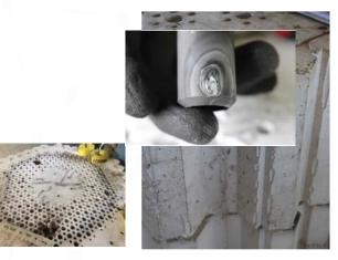
Damaged ceramic core block resulting from block shifting that degraded heater rod electrical continuity causing localized hot spots - 4 need to be replaced
