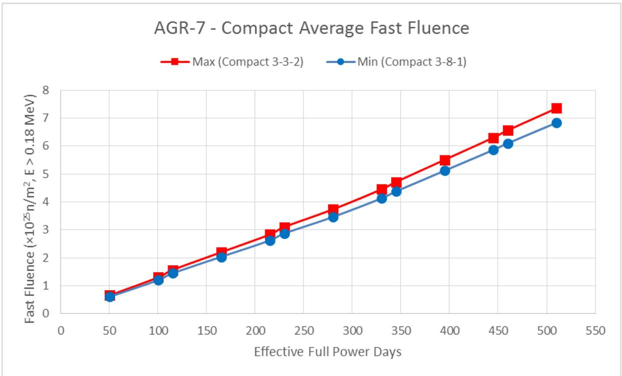
Figure 24. AGR-5/6 (top) and AGR-7 (bottom) minimum and maximum compact average fast neutron fluences.
