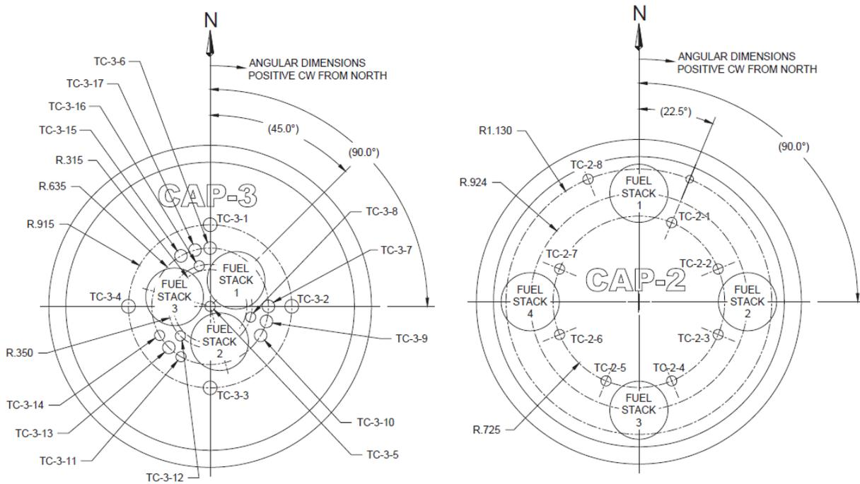
Figure 6. Cross sections of AGR-5/6/7 Capsules 3 (left) and 2 (right) showing the position of the TCs.
