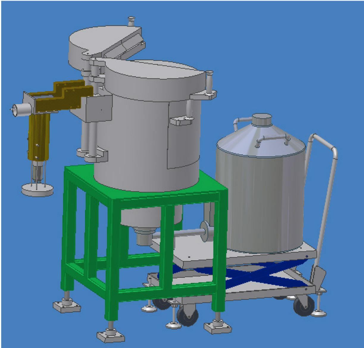
Figure 13. Gross radiation monitor and spectrometer detector for one AGR-5/6/7 sweep gas line.
