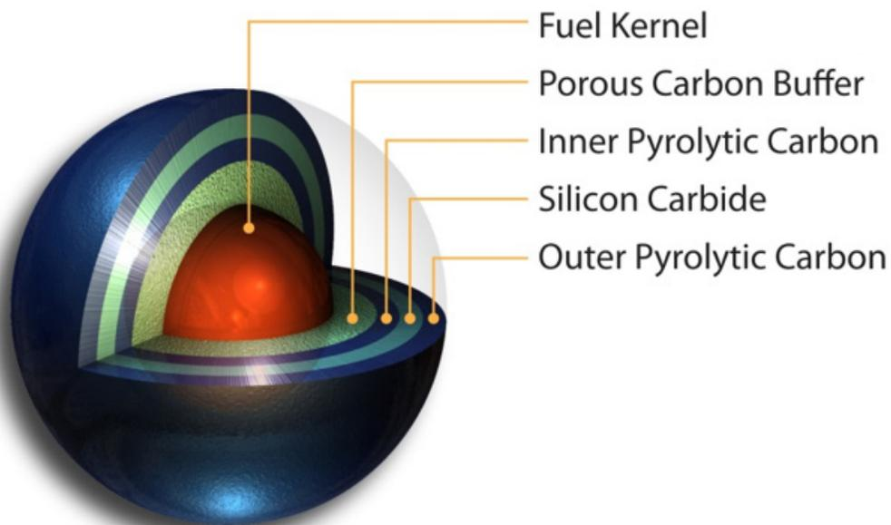
Figure 3. Graphic of a typical TRISO-coated fuel particle.
