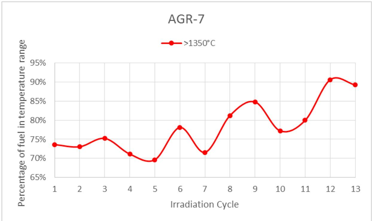
Figure 15. Percentage of the fuel in the AGR-5/6 (top) and AGR-7 (bottom) temperature ranges.
