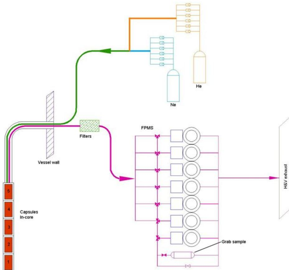
Figure 10. Simplified flow path for AGR-5/6/7 sweep gas.
