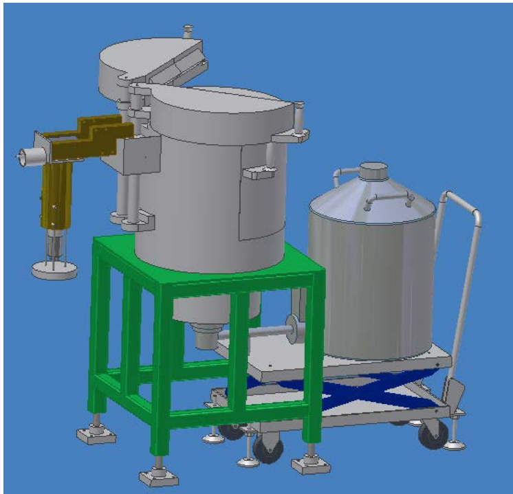
Figure 9. Gross radiation monitor and spectrometer detector for one AGR-3/4 sweep gas line.
