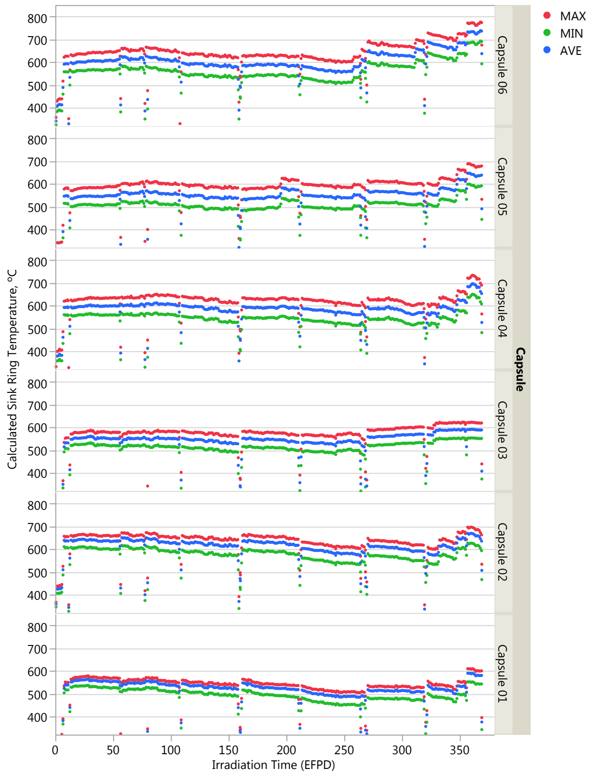
Figure C-10. Calculated daily minimum, maximum, and volume-average graphite sink temperatures for Capsules 1–6.
