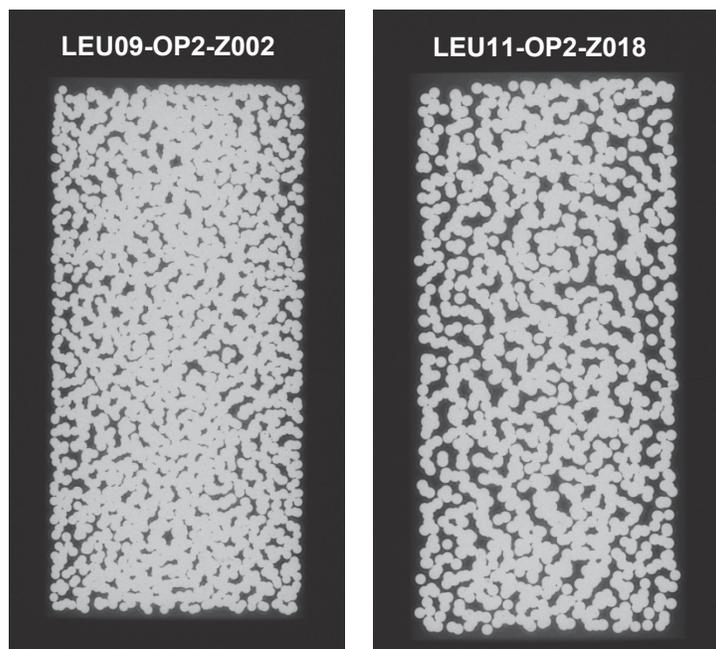
Figure 1. X-radiographs of U.S. UCO (compact LEU09-OP2-Z002, left) and UO<sub>2</sub> (compact LEU11-OP2-Z018, right) compacts taken from the same compact lots used in the AGR-2 irradiation. Note the visibly lower packing fraction of the UO<sub>2</sub> compact. Images taken from Hunn et al. 2010.
