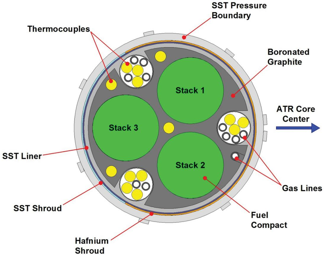
Figure 2. Cross-section diagram of an AGR-2 capsule (viewed from top).
