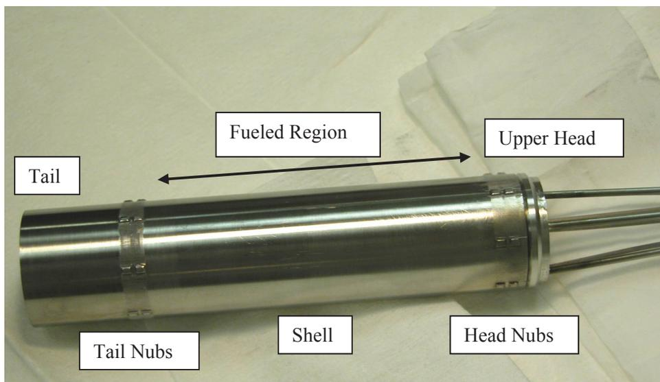
Figure 5. External configuration of an AGR-2 capsule.
