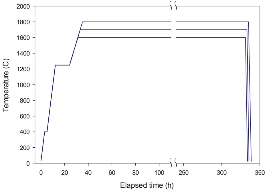
Figure 6. Temperature profiles for isothermal safety tests at maximum temperatures of 1600, 1700, and 1800°C.
