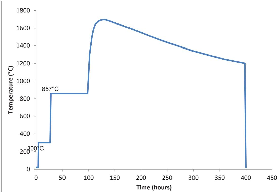
Figure 7. Proposed temperature profile for AGR-2 transient temperature accident simulation safety tests. Temperature profile based on that used for safety testing of German spherical fuel element AVR 91/31 (FZK report IWE-TN-17/93).
