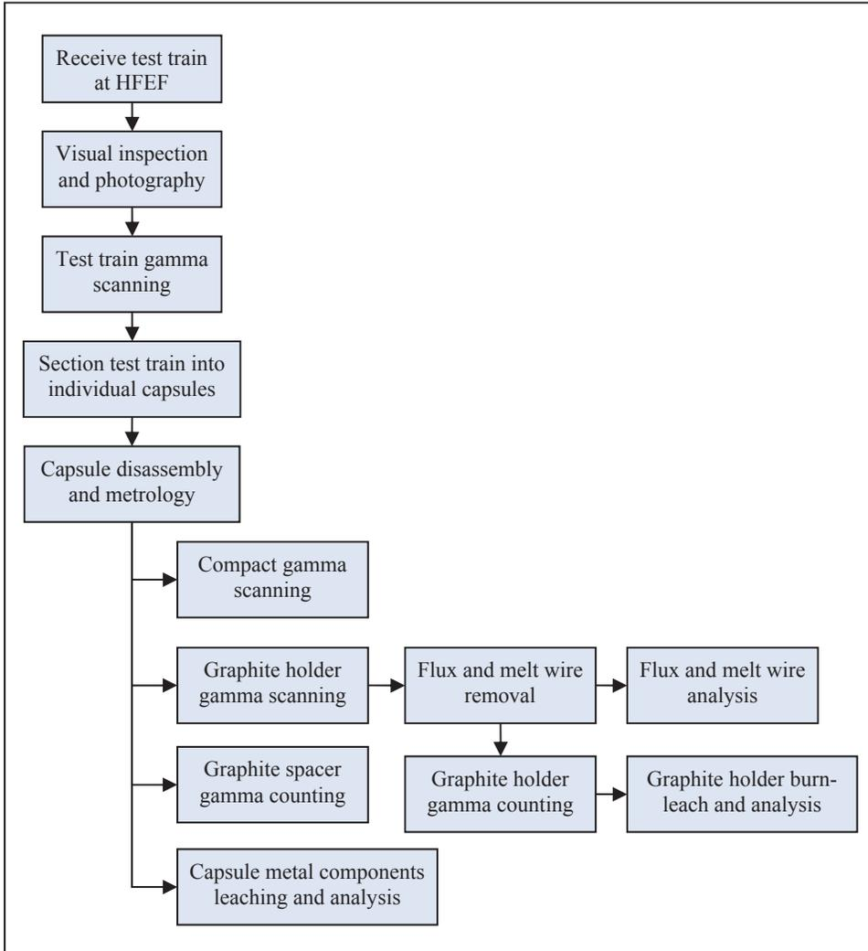
Figure 4. Flow diagram for AGR-2 test train inspection and disassembly, destructive examination of the capsule components, and non-destructive examination of the fuel compacts.
