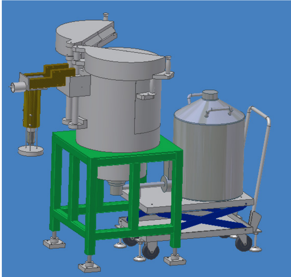
Figure 3-7. Gross radiation monitor and spectrometer detector for one AGR-2 sweep gas line.
