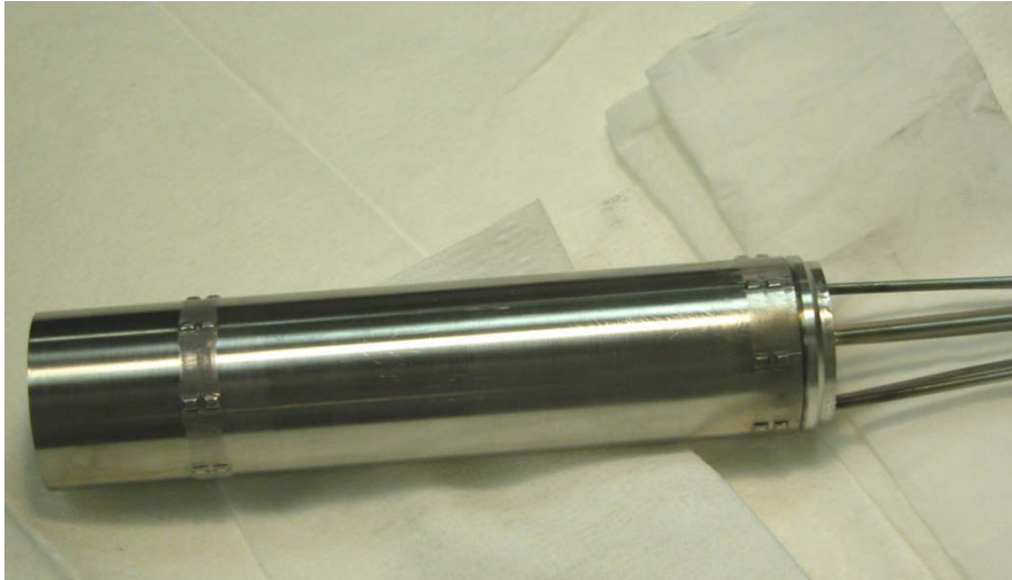
Figure 6. A single assembled AGR-1 capsule.
