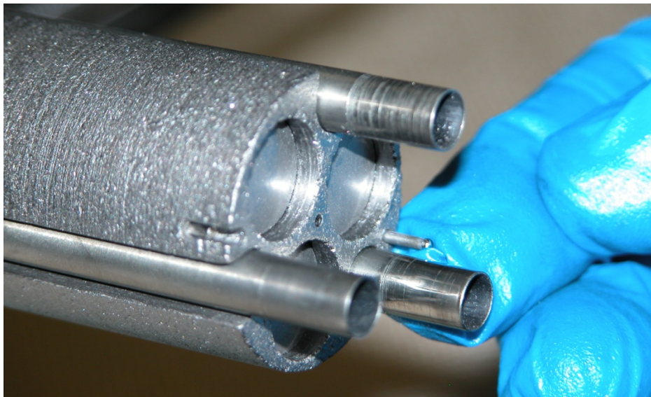
Figure 13. Flux wire package being inserted during capsule assembly activities.
