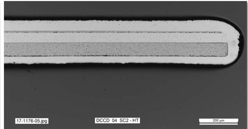
Cross-section of seal coated sample
