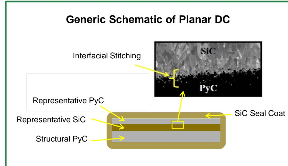
**First step in the process is to develop planar diffusion couple**
