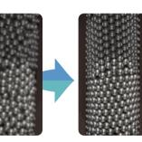
With increased computational resources, it is now possible to perform high-fidelity full-core simulation of pebble movements using Discrete Element Methods (DEM). Initially, the pebble bed packing of fuel spheres is random, with very few organized structures (*left*).
