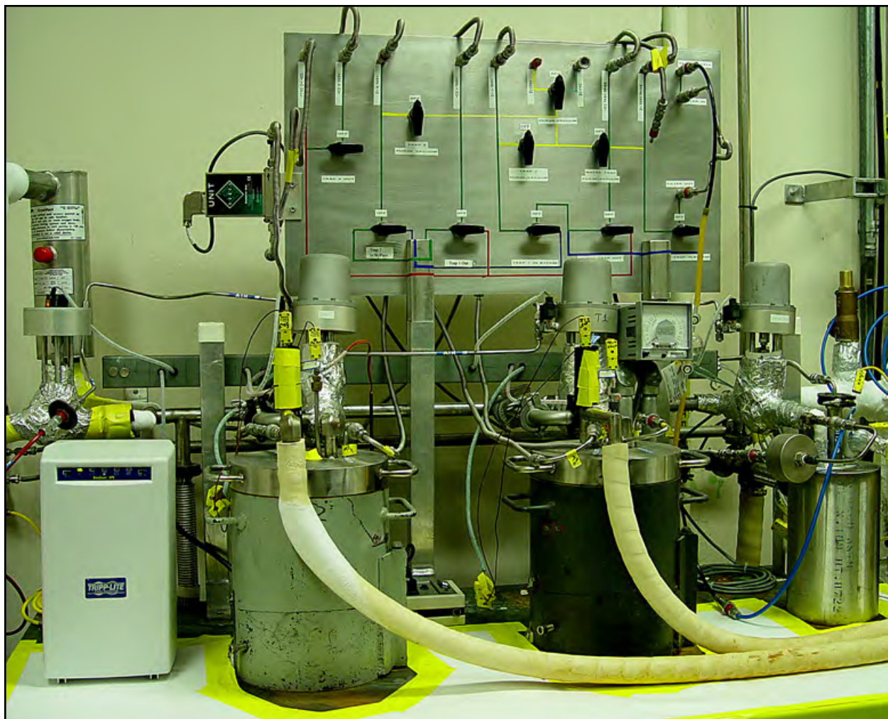
Appendix Figure A-3. CCCTF fission gas trap assembly.
