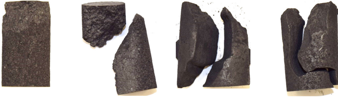
Figure 3. Trimmed samples showing failure modes more typical of virgin graphite.
