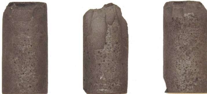
Figure 2. Preliminary untrimmed IG-430 samples showing failure at cylinder edges.
