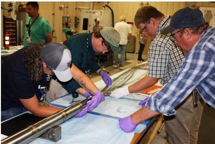
Assembly of AGR-5/6/7 in the test train assembly facility.
