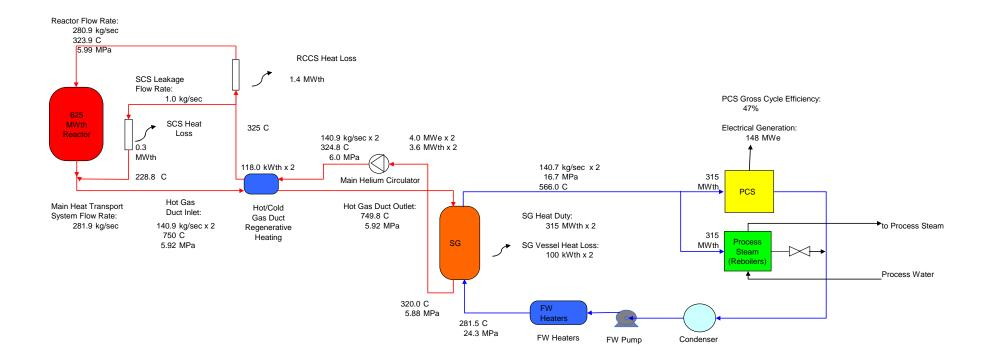
Figure 4-2: Heat Balance at Rated Power for 50%/50% Electricity Production and Process Heat Production
