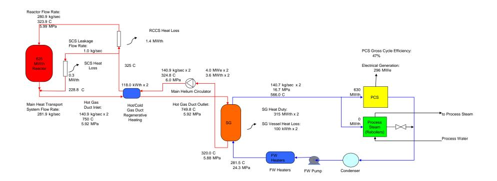
Figure 4-1: Heat Balance at Rated Power for 100% Electricity Production
