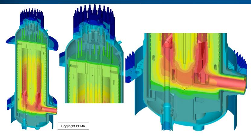
CFD modeling is employed to calculate detailed temperature distributions of the components. This is used downstream in the structural design.
