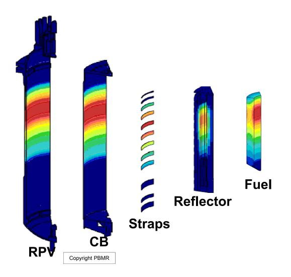
Heat is generated in both local (in the fuel) and nonlocal sources
