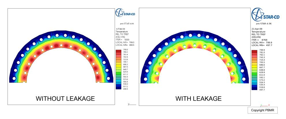
Increased thermal gradients impacts on the stresses in the components
