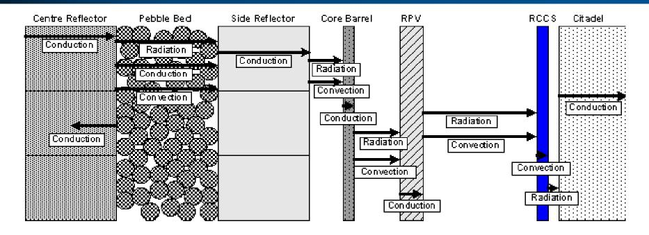
This path transfers the heat stored in the structures and the decay heat generated to the outside of the reactor vessel for removal to the environment, without exceeding component temperature limits
