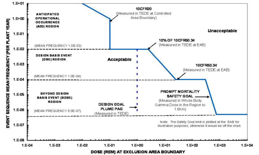
Design goal is to meet the EPA Protective Action Guideline (PAG) at 425m EAB rather than the 16,000m EPZ for existing LWRs
