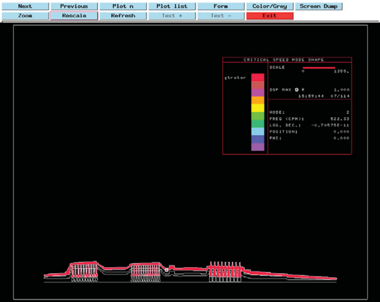
Figure 41 Flexible Bearings - First Forward Critical Speed 522rpm (11.9%N)
