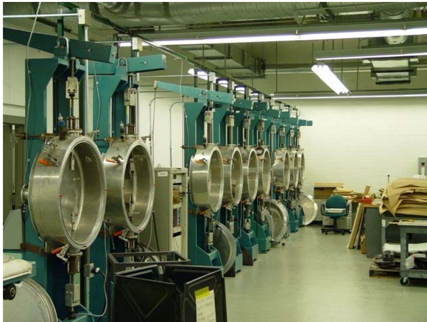
Fig. 9: Creep machines under preparation for negligible creep testing
