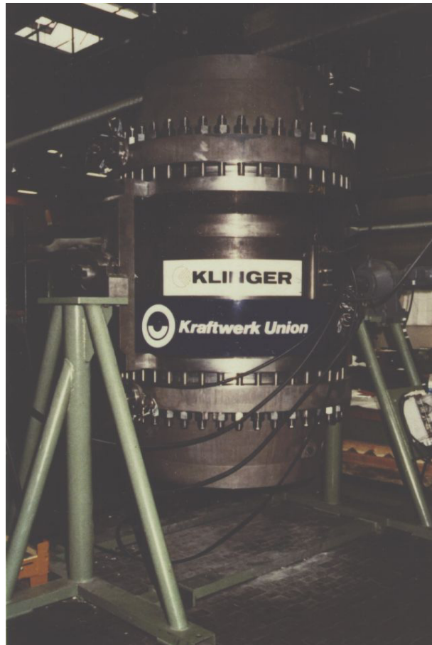
Figure 5-6 Manufacturing Isolation Valve
