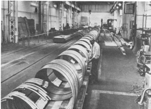
Figure 11-1: Helical Heat Exchanger Tube Test in KVK Loop
