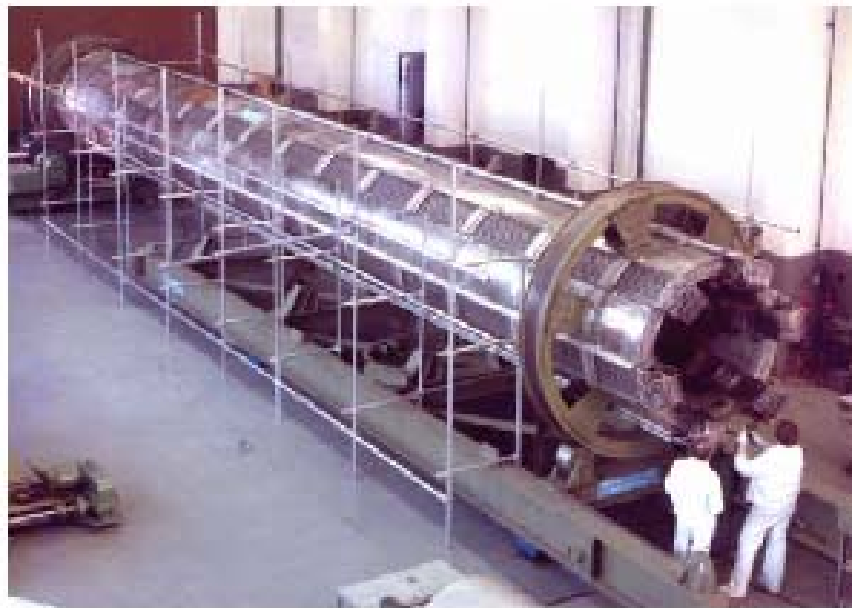
He-He intermediate heat exchanger before installation
