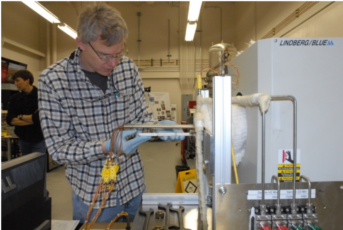
Figure 4. Insertion of specimen in alumina boats.
