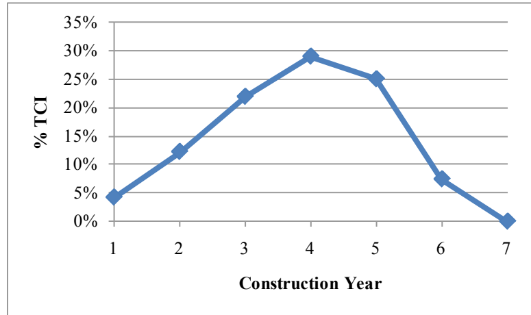
Figure 6. Percentage of TCI spent each year of construction, HTGR-integrated ex situ oil shale retorting.
