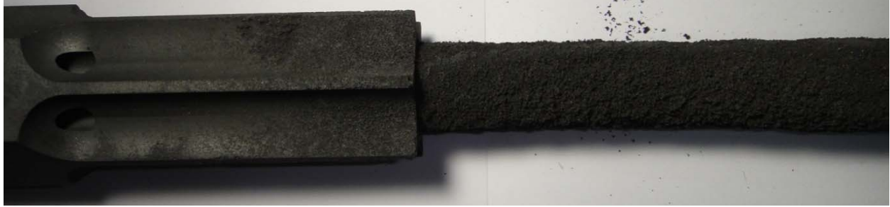
Figure 7-39. Oxidized graphite structure in the case with initial temperature of 650°C.
