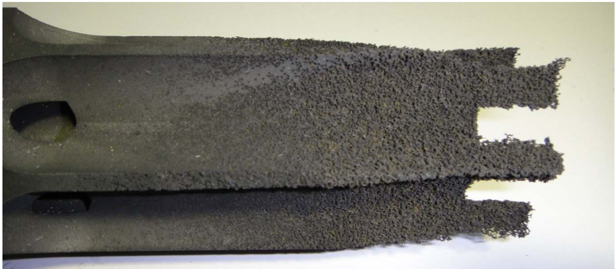
Figure 7-40. Oxidized graphite structure in the case with initial temperature of 1050°C.
