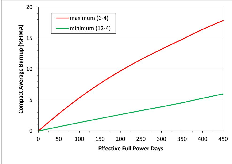
Figure 4-4. Compact average burnup for the maximum compact (Capsule 6 – Level 4) and minimum compact (Capsule 12 – Level 4).
