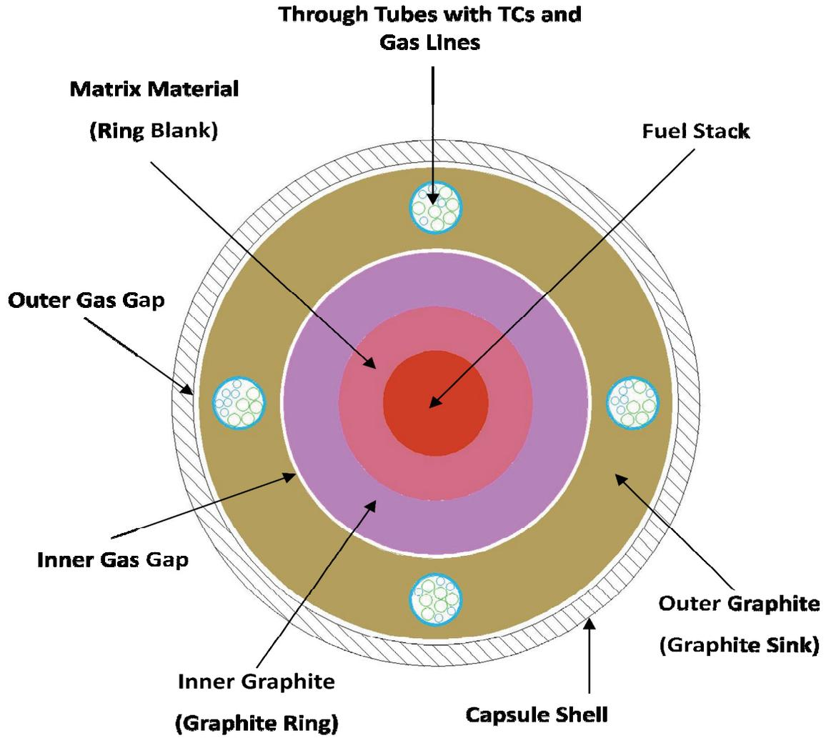
Figure 3-4. Radial schematic of an AGR-3/4 capsule.
