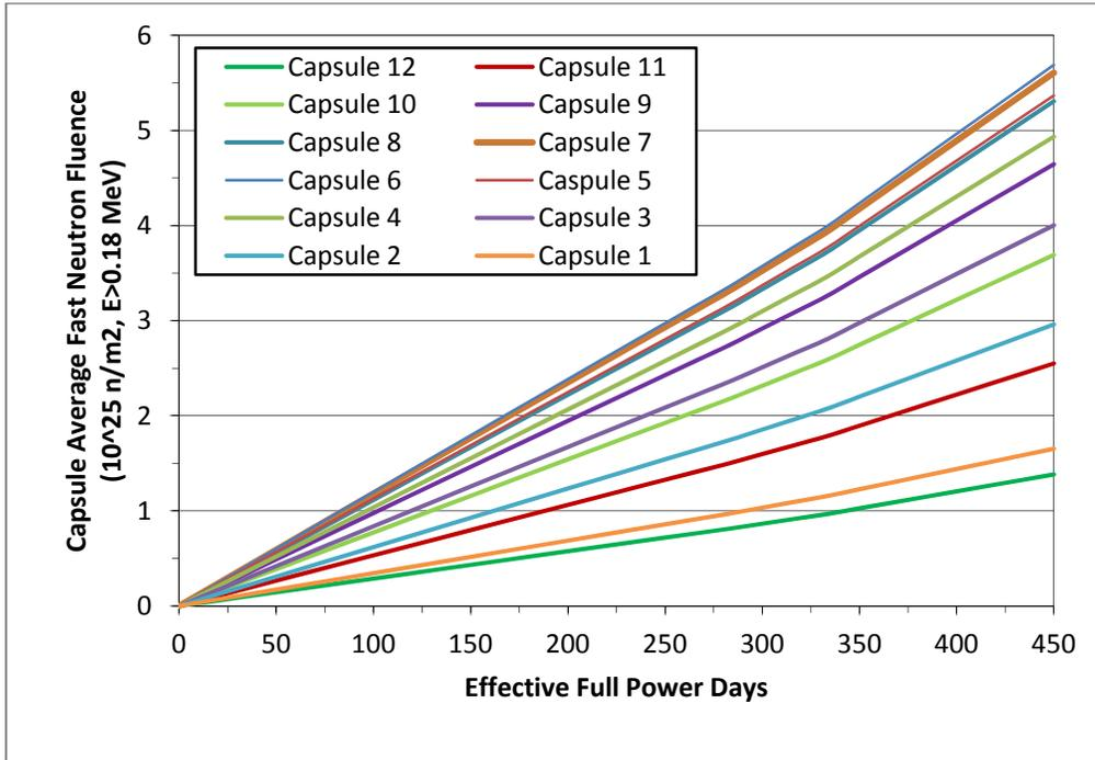
Figure 4-5. Capsule average fast neutron fluences for AGR-3/4.
