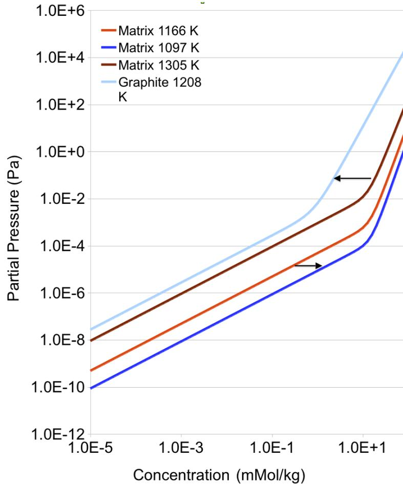
Figure 5-3. Cesium sorption isotherms at AGR-3/4 conditions.
