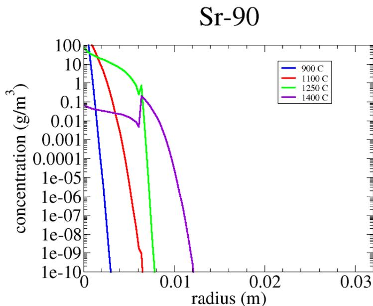
Figure 5-6. Sr-90 concentration profiles at 300 EFPD.
