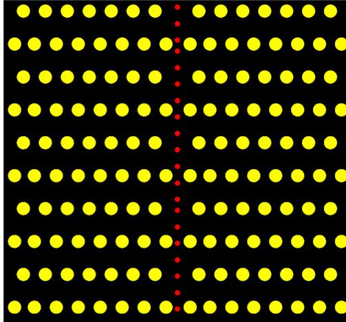
Figure 3-2. Schematic of an AGR-3/4 compact with DTF fuel particles placed along the axis.
