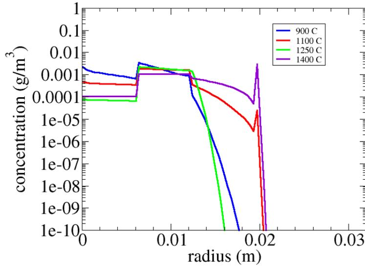
Figure 5-4. Ag-110m concentration profiles at 300 EFPD.
