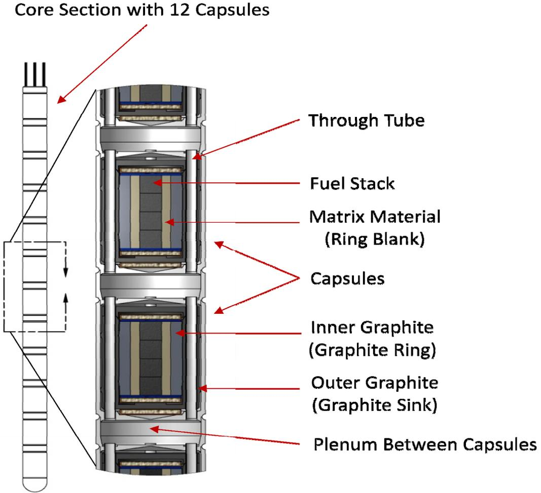
Figure 3-3. Axial schematic of the AGR-3/4 capsules.
