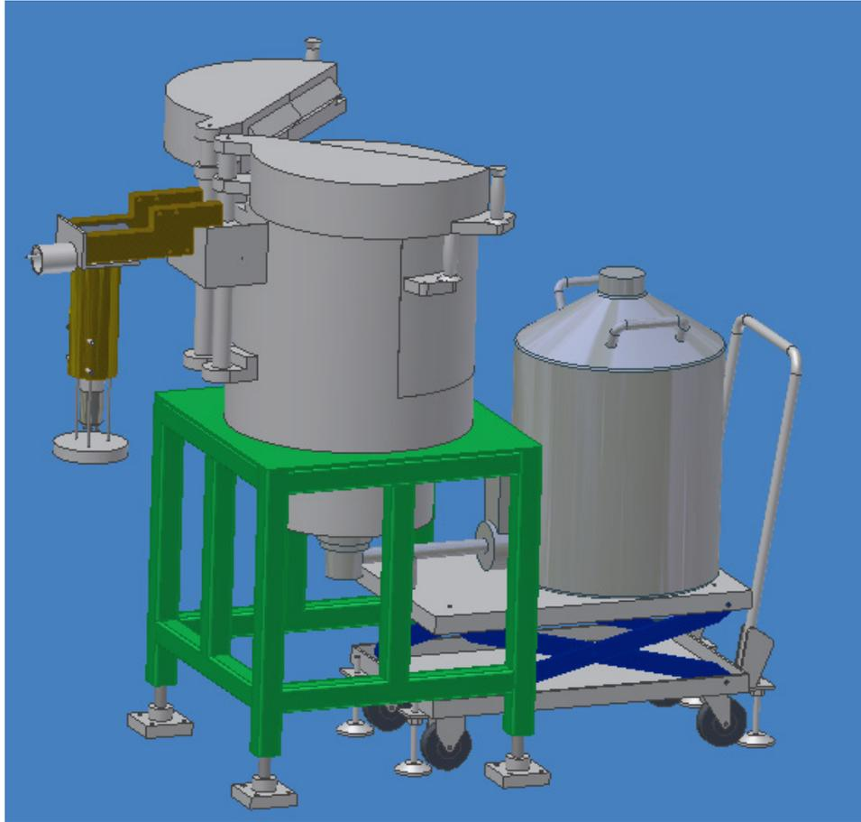
Figure 3-8. Gross radiation monitor and spectrometer detector for one AGR-3/4 sweep gas line.
