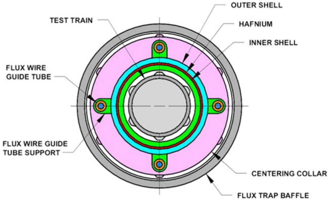
Figure 3-6. Radial schematic of the AGR-3/4 irradiation housing.
