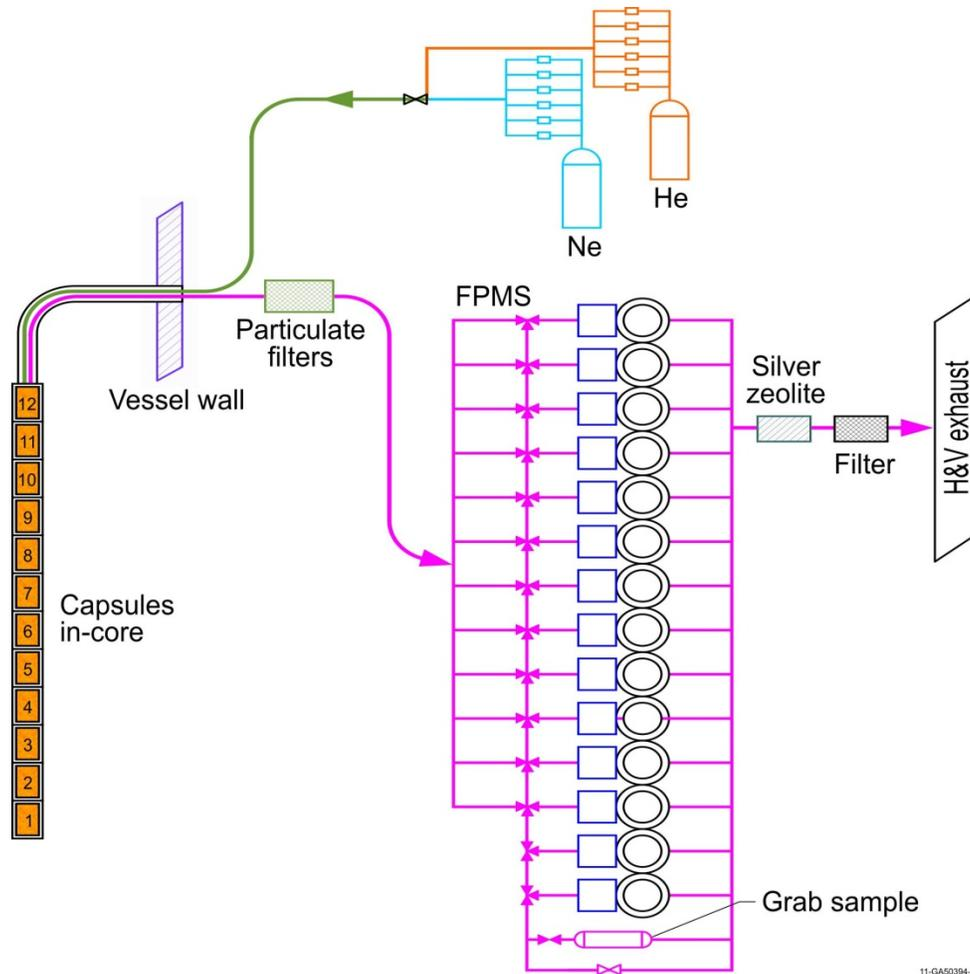
Figure 3-5. Simplified flow path for AGR-3/4 sweep gas.
