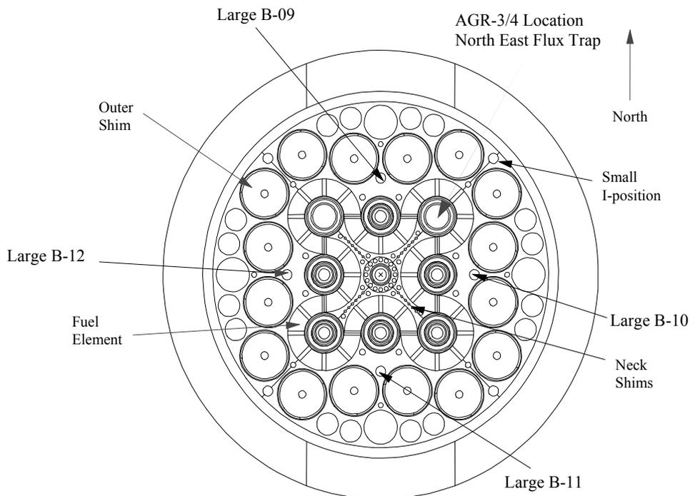
Figure 2-1. ATR core cross section displaying the NEFT position.
