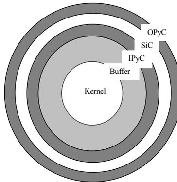
Figure 3-1. Schematic of a typical TRISO-coated fuel particle.
