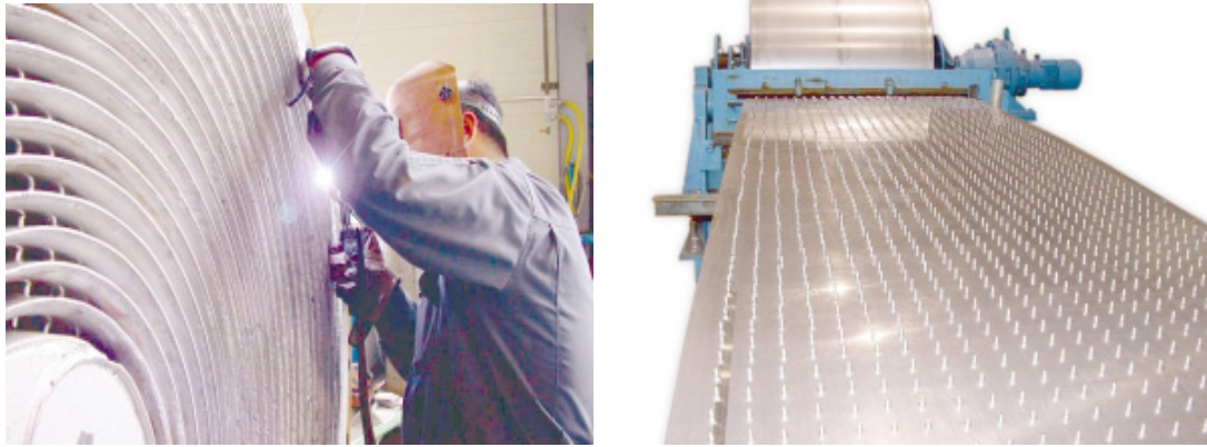
Figure 5-20. Manufacturing of a SHE (Fisher and Sindelar 2008).
