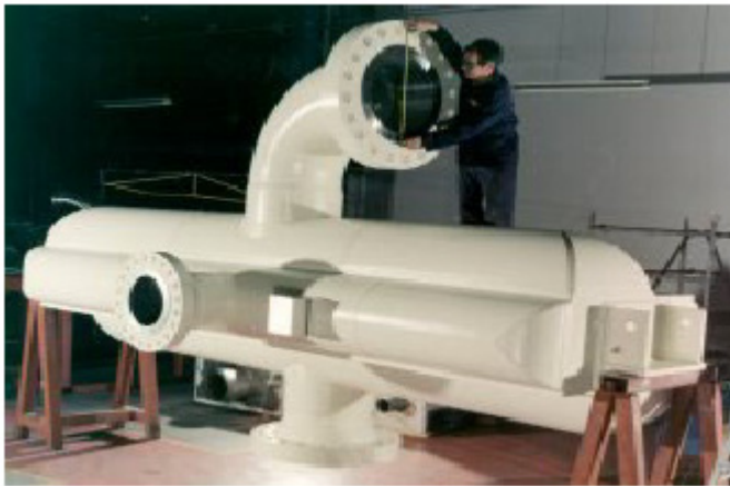
Figure 5-13. Finished heat exchanger (Heatric™ Homepage 2007).
