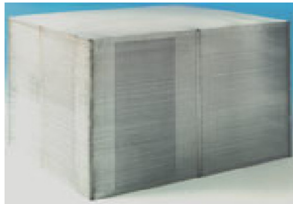
Figure 5-10. Third step - block composed of diffusion bonded plates (Heatric™ Homepage 2007).
