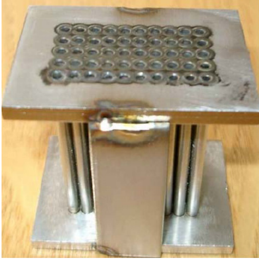
Figure 2-9. Capillary heat exchanger mock-up.
