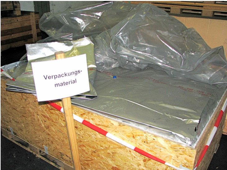
Figure 4. Photos of prospective packaging for NBG-18 transatlantic shipment. The blue nozzle allows backfilling of the vapor barrier with an inert gas.
