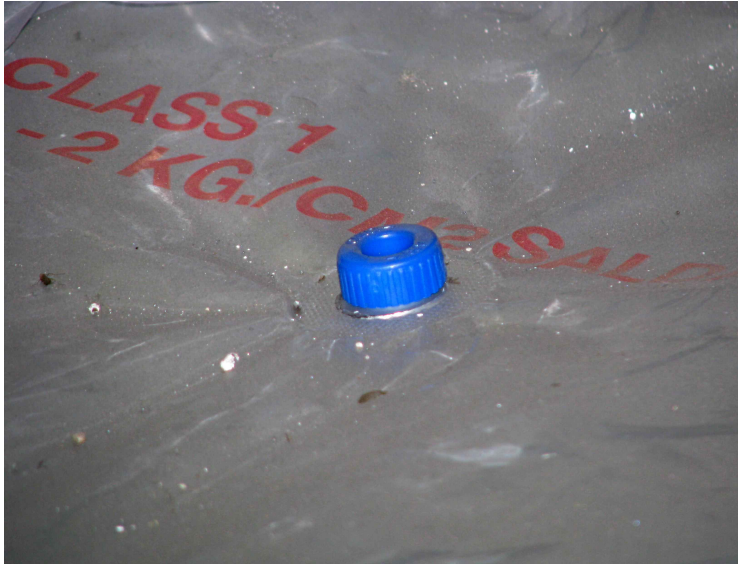
Figure 5. Photos of prospective packaging for NBG-18 transatlantic shipment. The blue nozzle allows backfilling of the vapor barrier with an inert gas.
