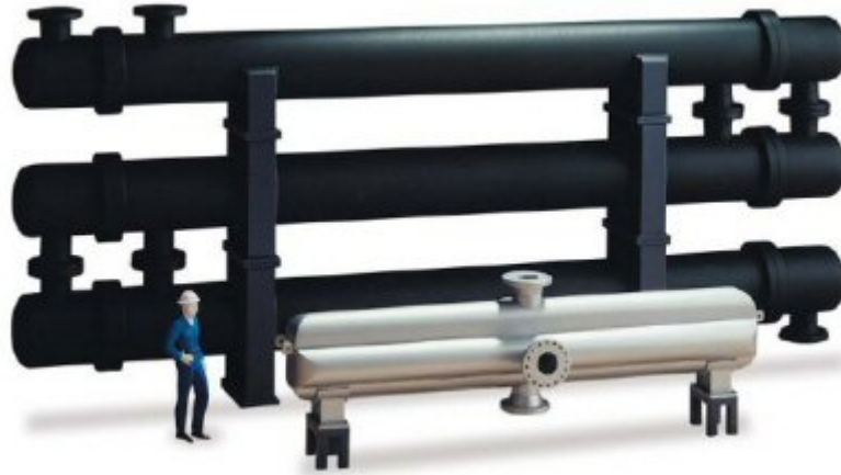
Figure 3. The diffusion-bonded heat exchanger in the foreground undertakes the same thermal duty, at the same pressure drop, as the stack of three shell and tube exchangers behind.
