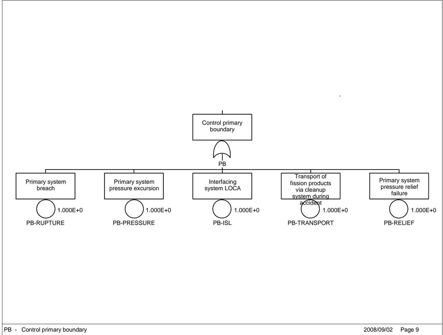
Figure 5. Master Logic Diagram for the NGNP – Control of primary boundary
