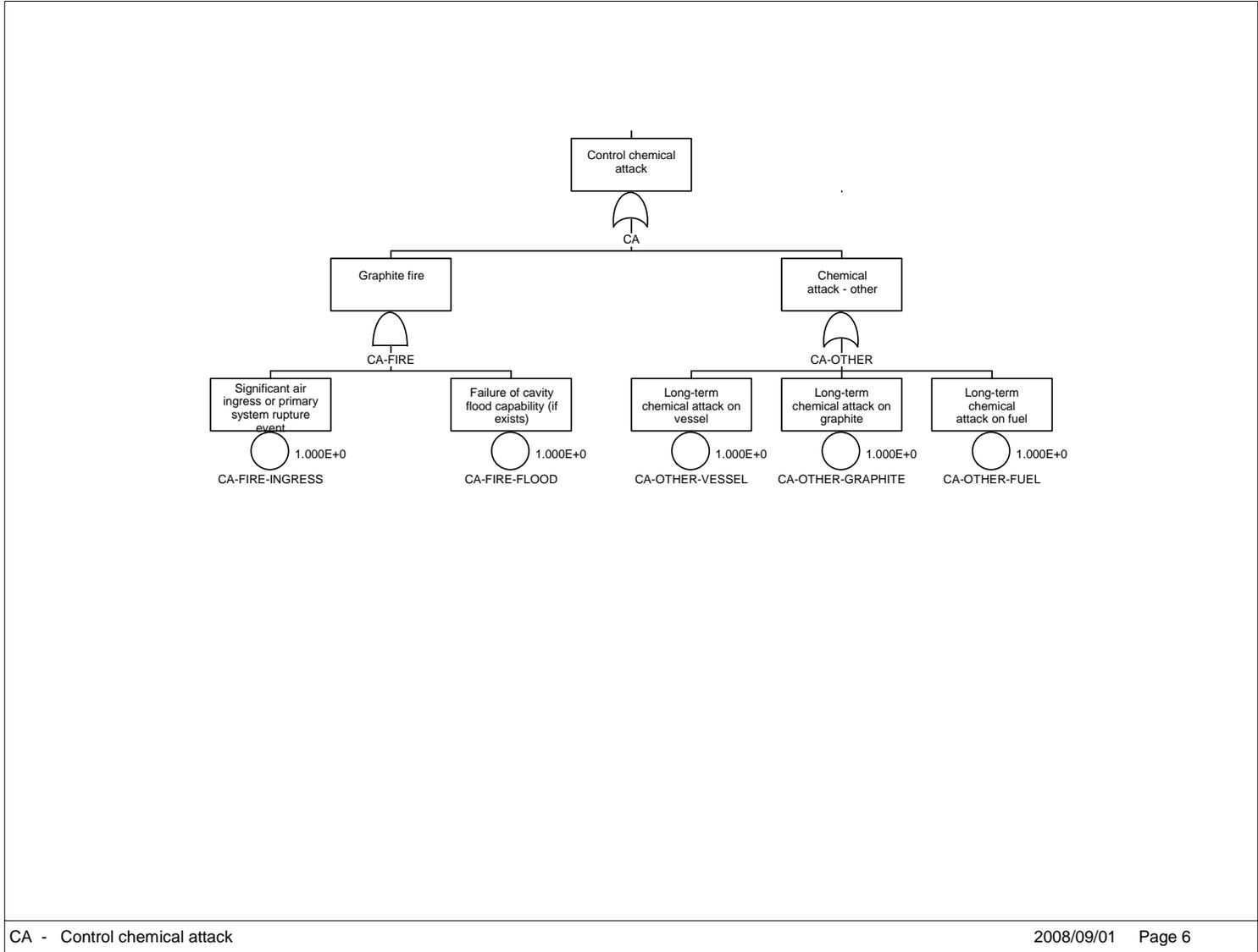
Figure 2. Master Logic Diagram for the NGNP – Control of chemical attack
