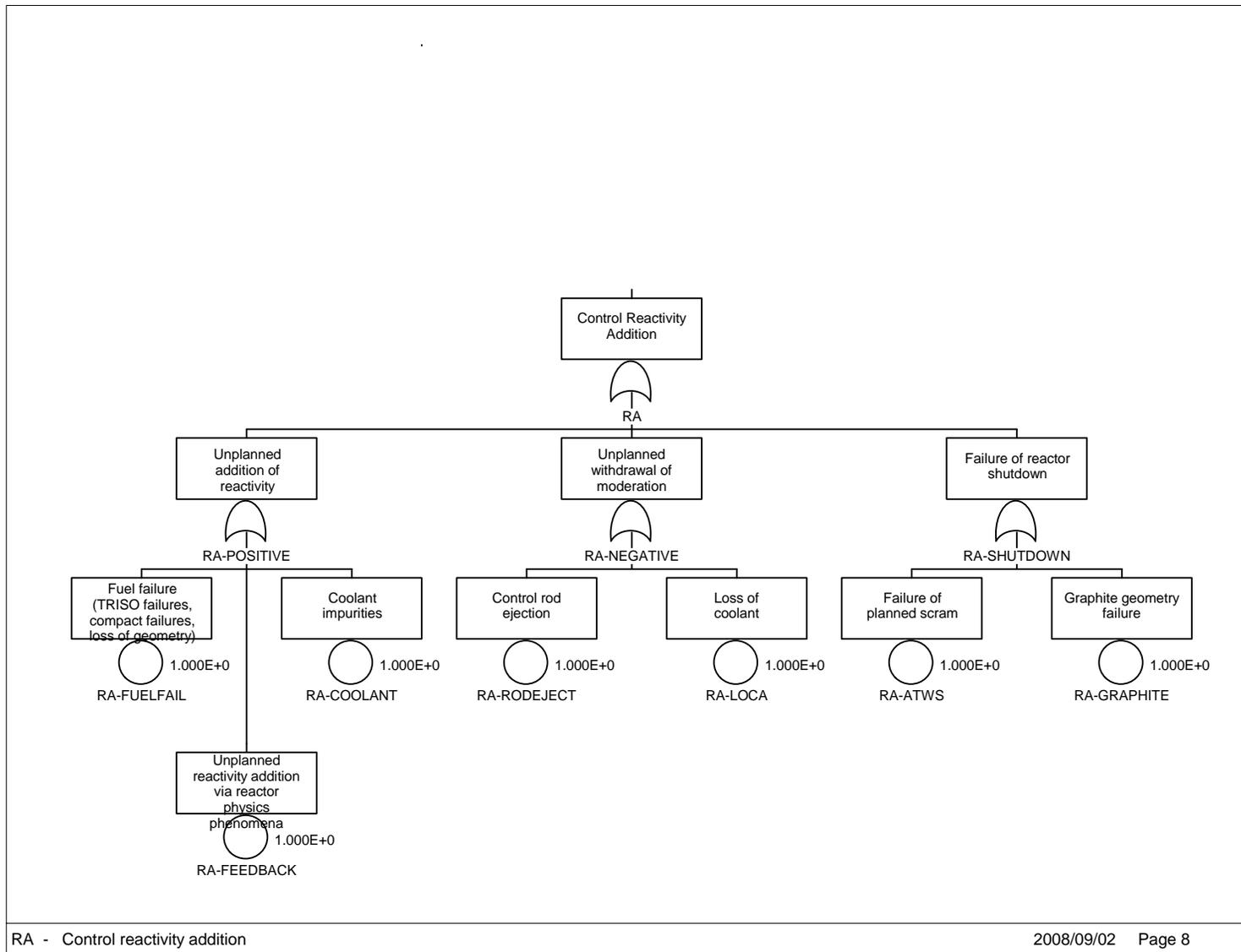
Figure 6. Master Logic Diagram for the NGNP – Control of reactivity addition
