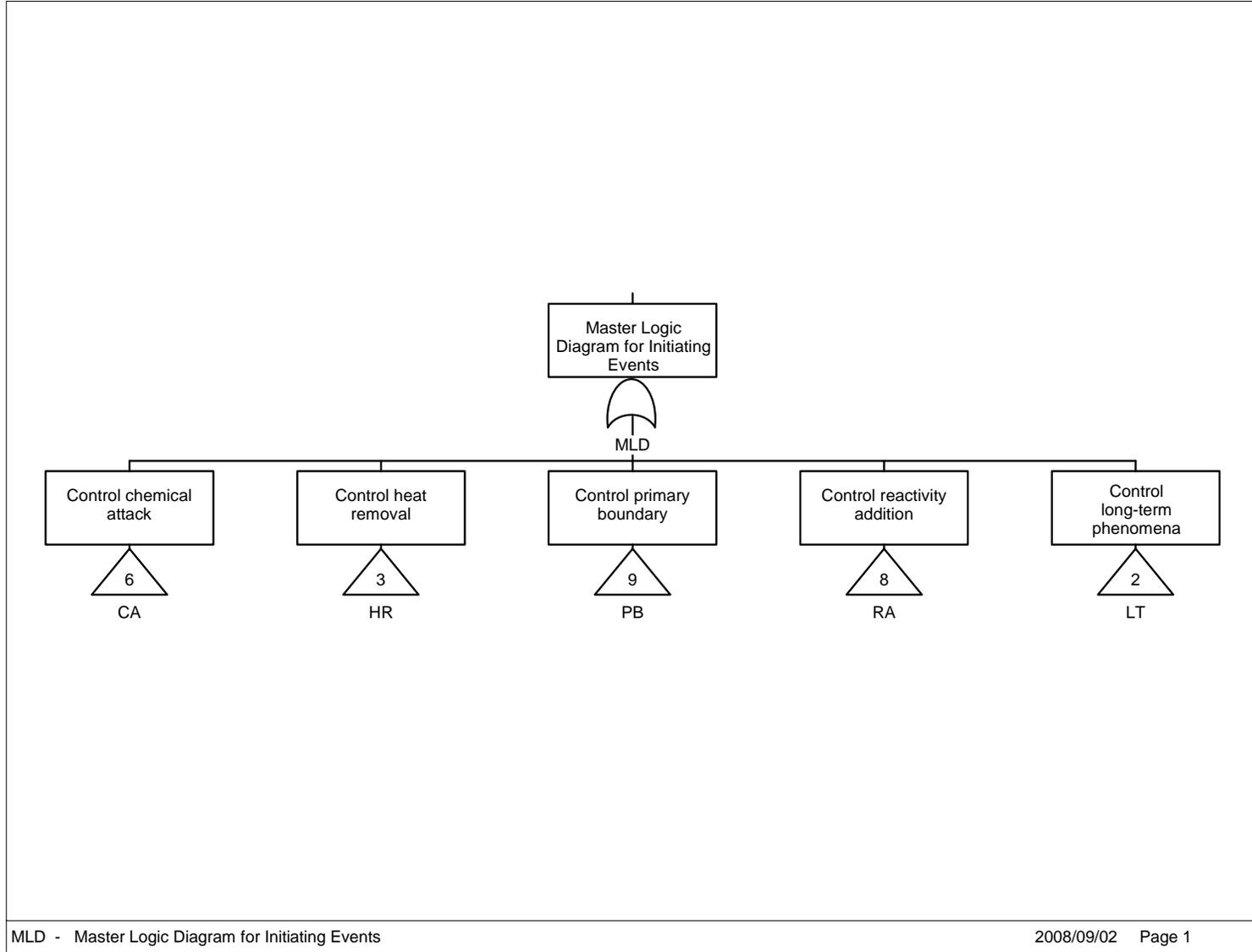
Figure 1. Master Logic Diagram for the NGNP
