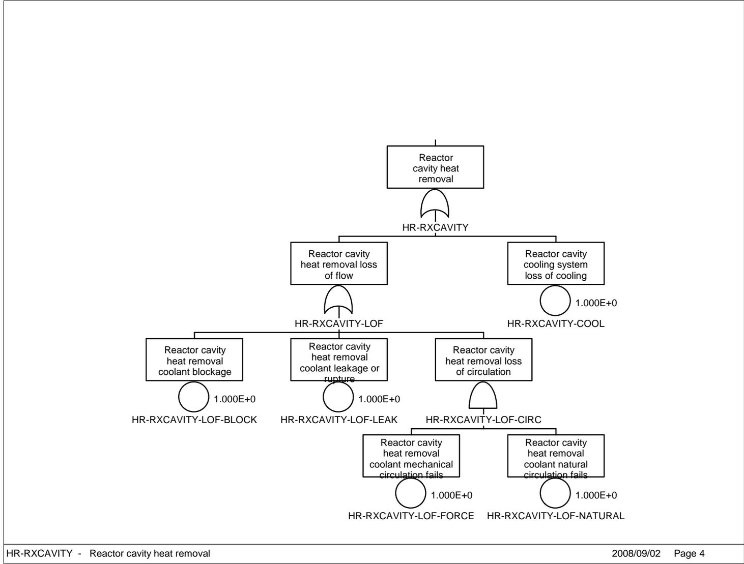
Figure 4. Master Logic Diagram for the NGNP – Control of heat removal (continued)
