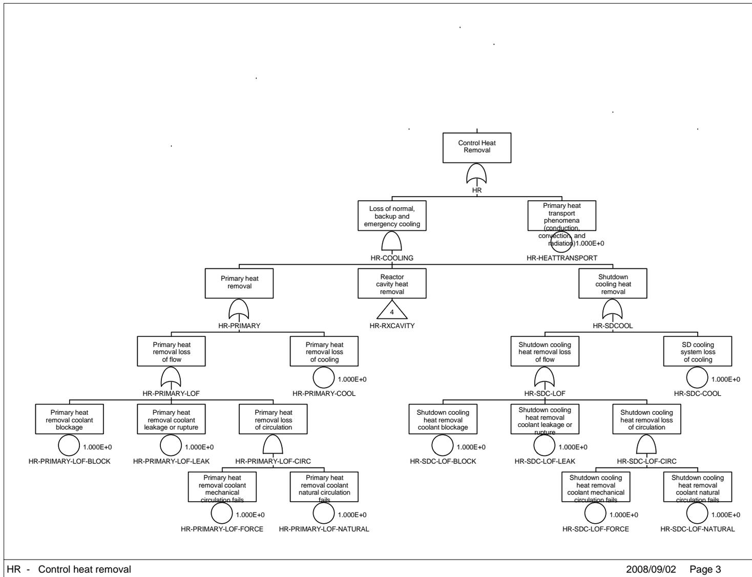
Figure 3. Master Logic Diagram for the NGNP – Control of heat removal
