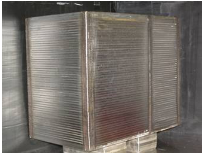
Figure 11. Heatric diffusion-bonded compact plate heat exchanger block.
