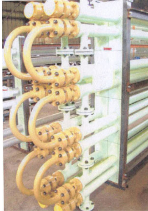
Figure 8. Hairpin heat exchangers manufactured by Brown Fintube France S.A.
