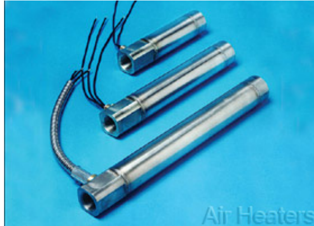
Figure 22. In-line air heaters operate up to 700°C and 120 psig (Heat Torch™ 200 by Farnum Custom Products, Inc.).
