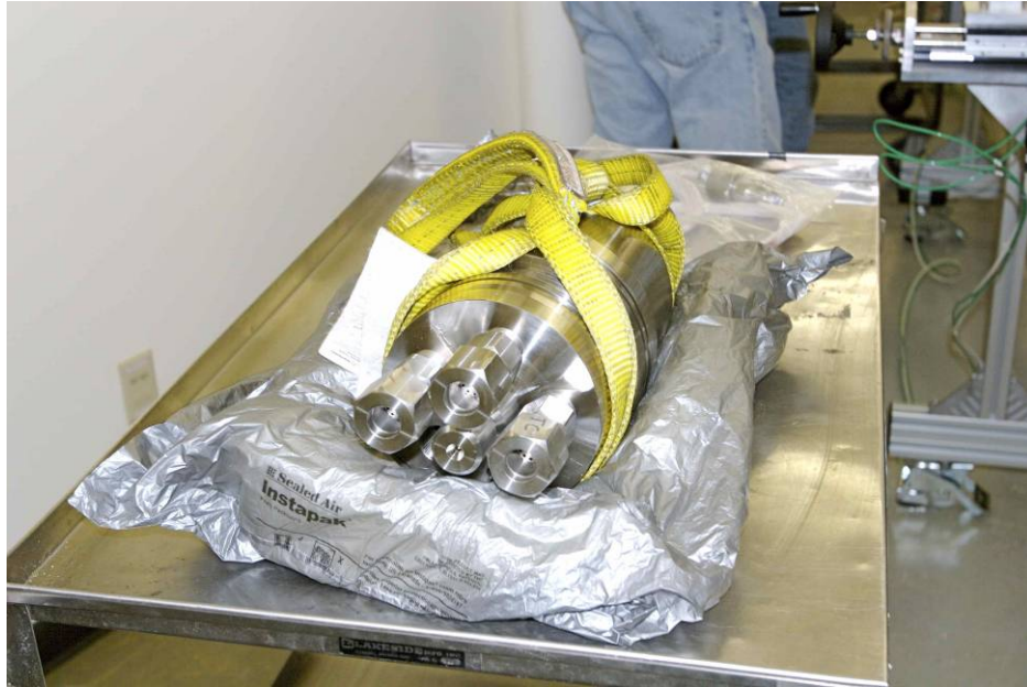
Figure 28. Completed upper head closure with Conax seals installed.
