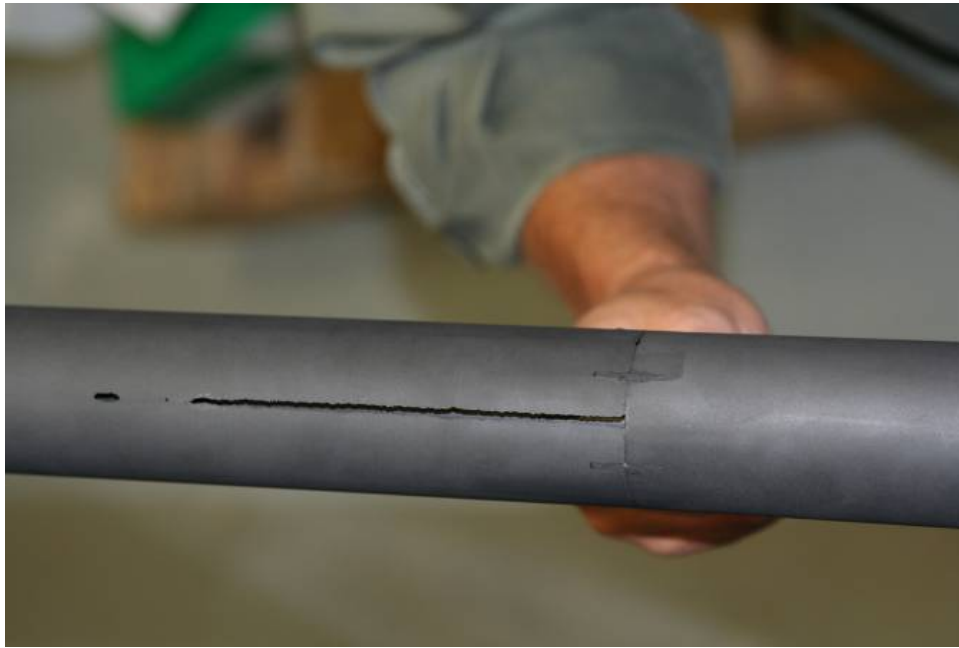
Figure 5. Machining defect on the upper core graphite body.
