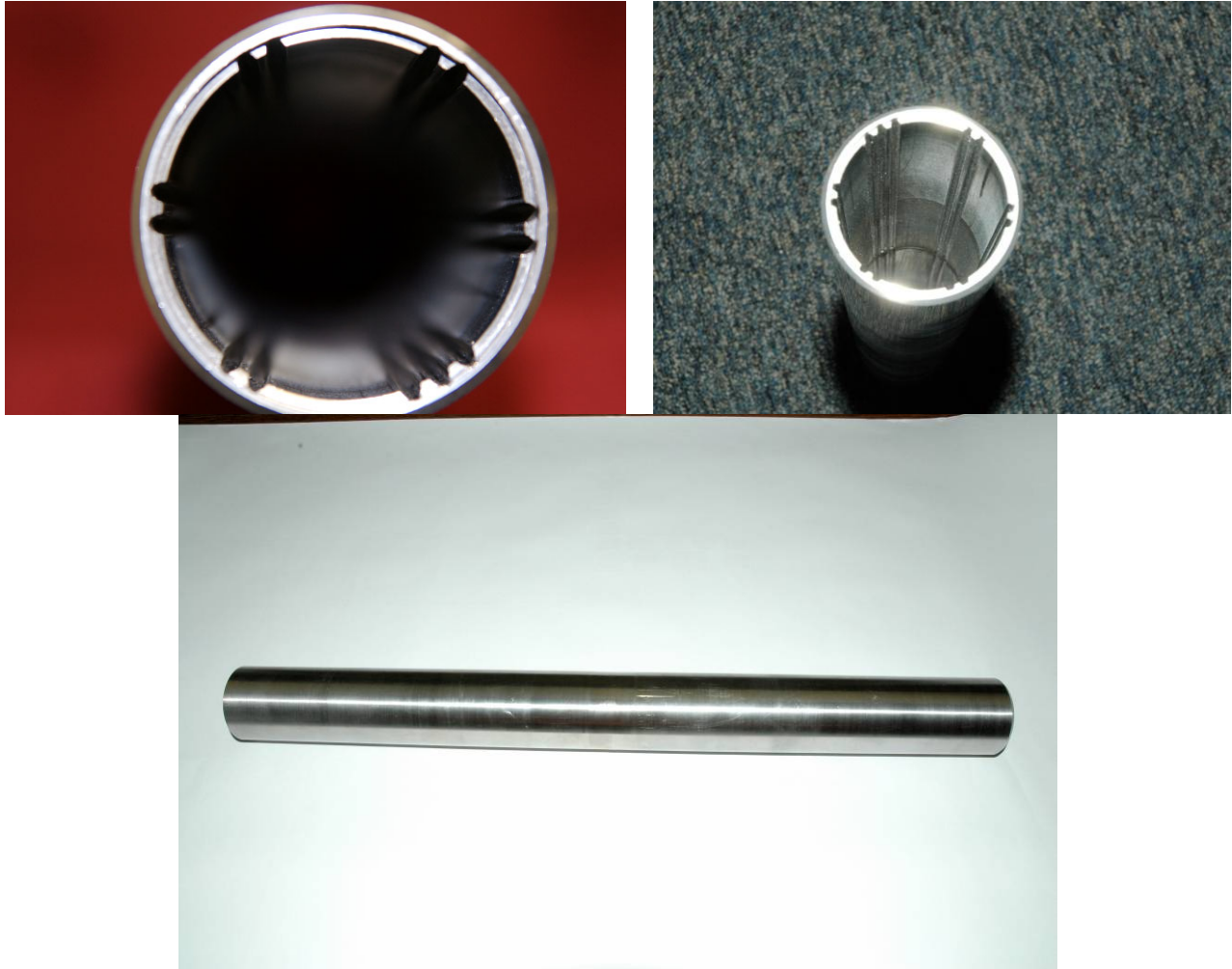
Figure 15. Completed 2-ft outer pressure boundary scoping test.
