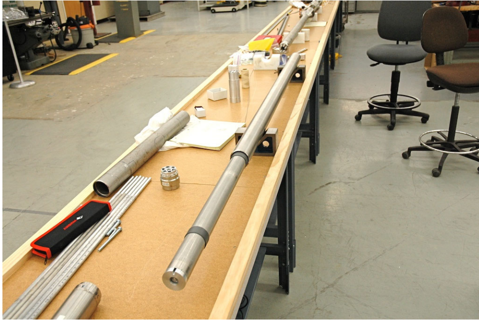
Figure 24. Loading the heat shield into the broached outer pressure boundary.
