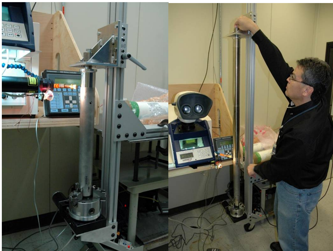
Figure 10. Set up for laser welding on the heat shield.
