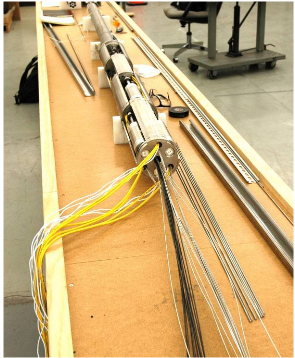
Figure 26. Installation of thermocouples and gas lines in the upper section of the mockup.
