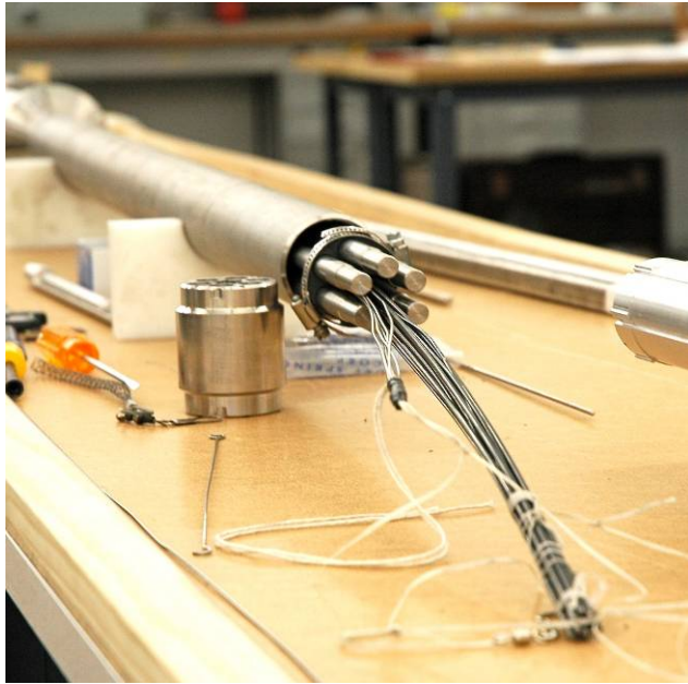
Figure 26. Installation of thermocouples and gas lines in the upper section of the mockup.
