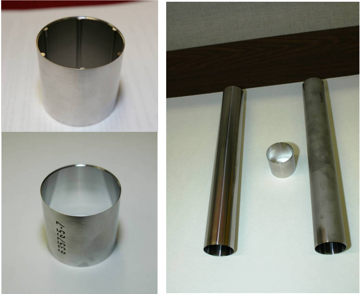
Figure 9. Delivered Haynes 230 heat shield parts.
