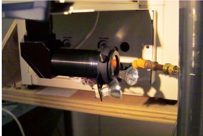
Figure 12. Right angle lens installed on the laser welder.
