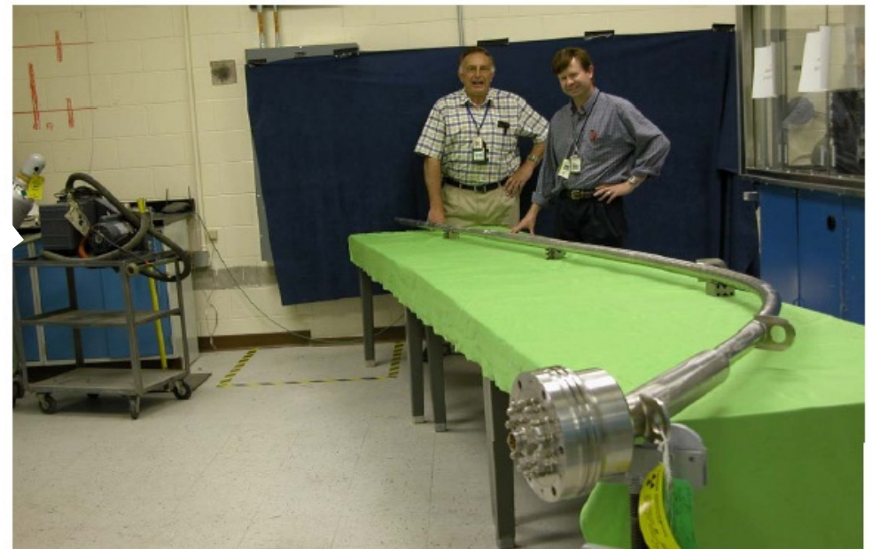
AGR-1 test train assembly 6-individual instrumented capsules
