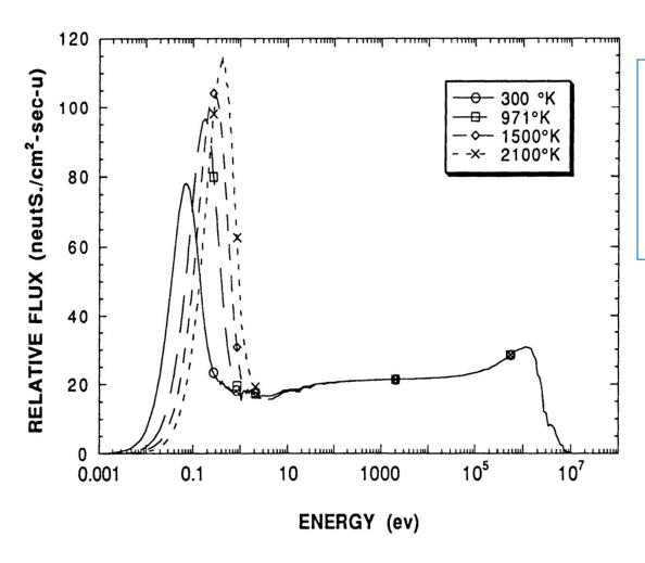
As core temperature Increases, the flux spectrum moves into the U-238 and Pu-240 resonance absorption cross section range.
