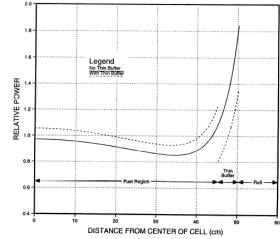
Reflector control rods are used for reactivity control during normal operation, and the control sequence is varied for more uniform burnup, and control of power peaks
