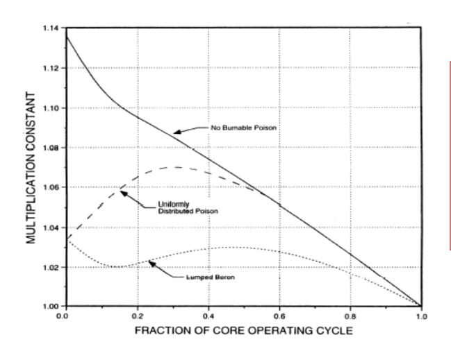
Self shielding of the lumped boron (B4C) used to control poison burnout and core reactivity behavior over a fuel cycle to minimize control rod requirements
