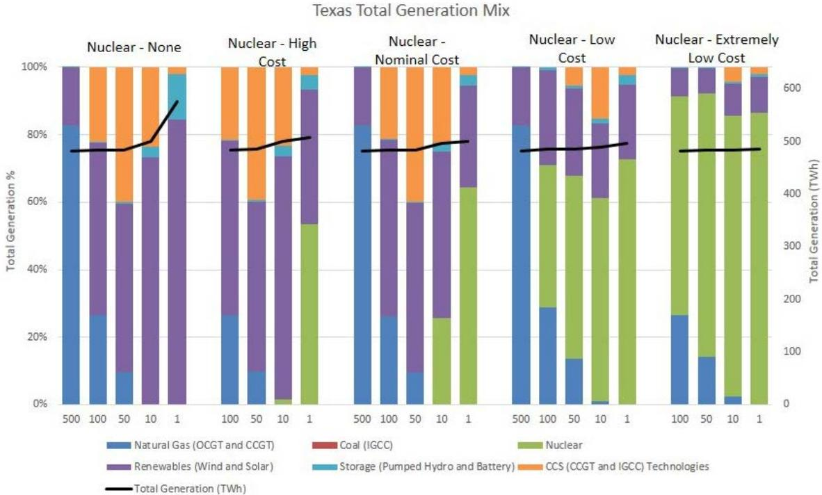
Fig. 5.1.a. Texas Total Generation Mix (left) and Total Generation (right; black line) versus Carbon Dioxide Constraint
