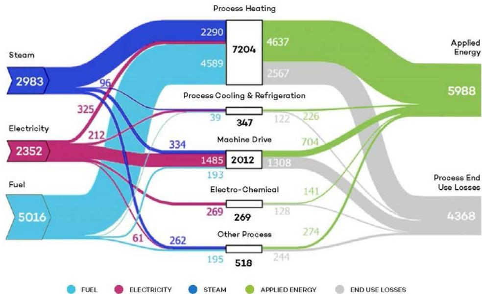
Fig. 7.6. U.S. Manufacturing Process Energy Flows in 2010: TBTU (U.S. DOE 2010, Breakthrough Institute 2019)
