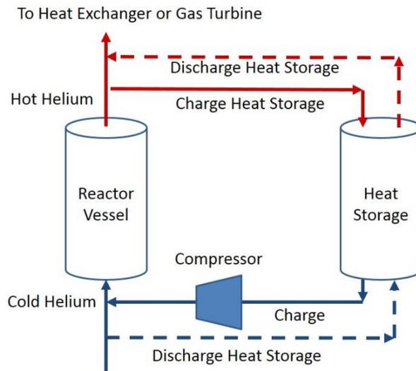
Fig. D.1. HTGR with At-Pressure Heat Storage
