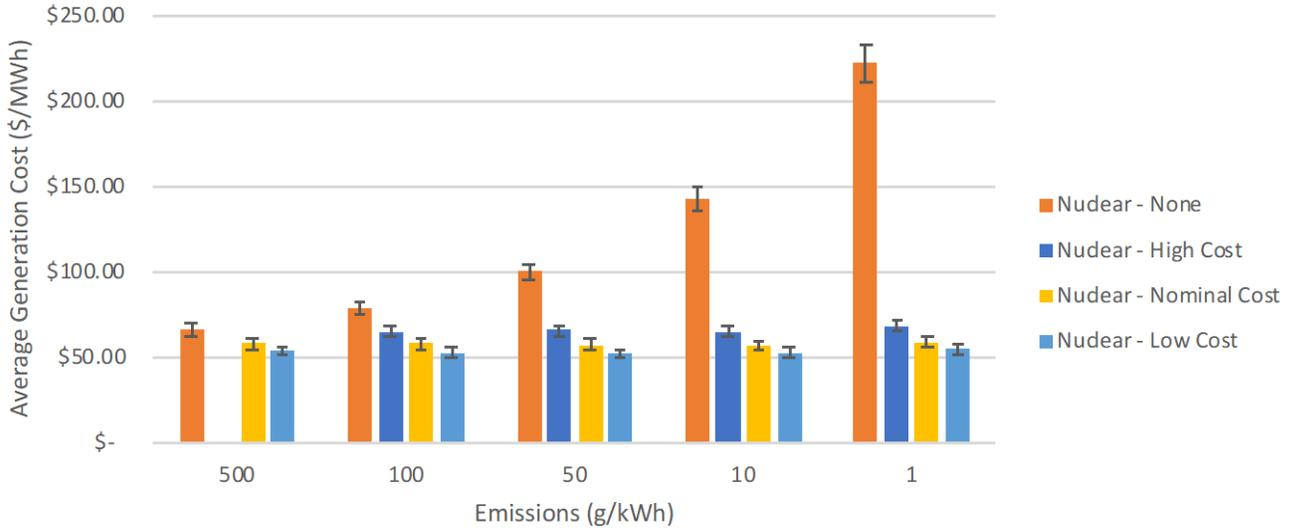
Figure 3.1.c: T-B-T Cost of Electricity Generation<sup>5</sup>
