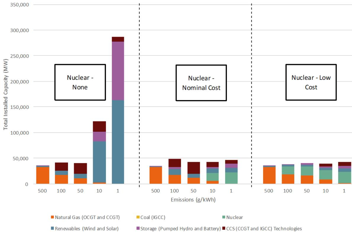
*Figure 4.2.b: Optimal Capacity Mixes for New England*
