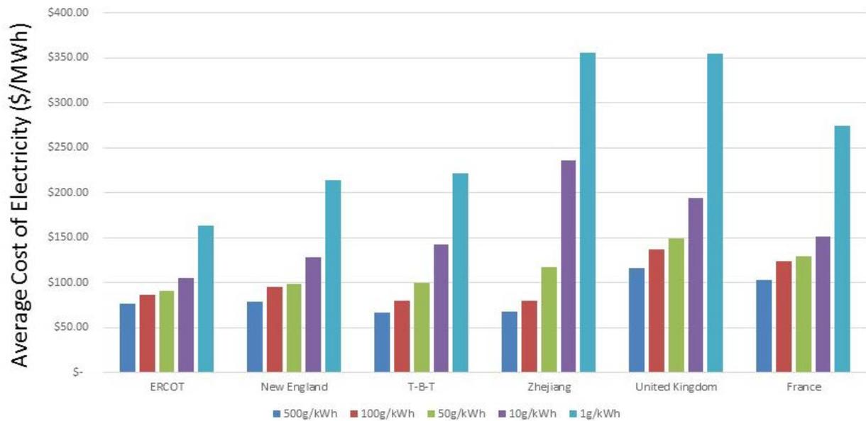
Fig. S.2. Average Cost of Electricity for Non-Nuclear Scenarios versus Carbon Constraint
