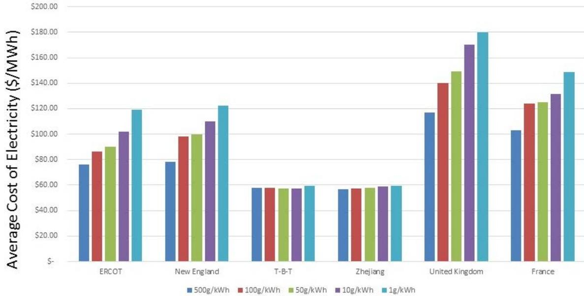
Fig. S.1. Average Cost of Electricity (All Technologies Allowed) Versus Carbon Constraint
