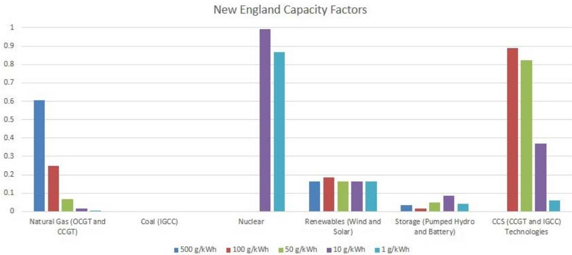
Fig. 6.1.b. Capacity Factors of Generating Technologies in New England versus CO<sub>2</sub> Emission Limits
