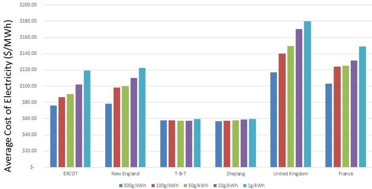
Figure 3.2. Average Cost of Electricity (All Technologies Allowed) Versus Carbon Constraint
