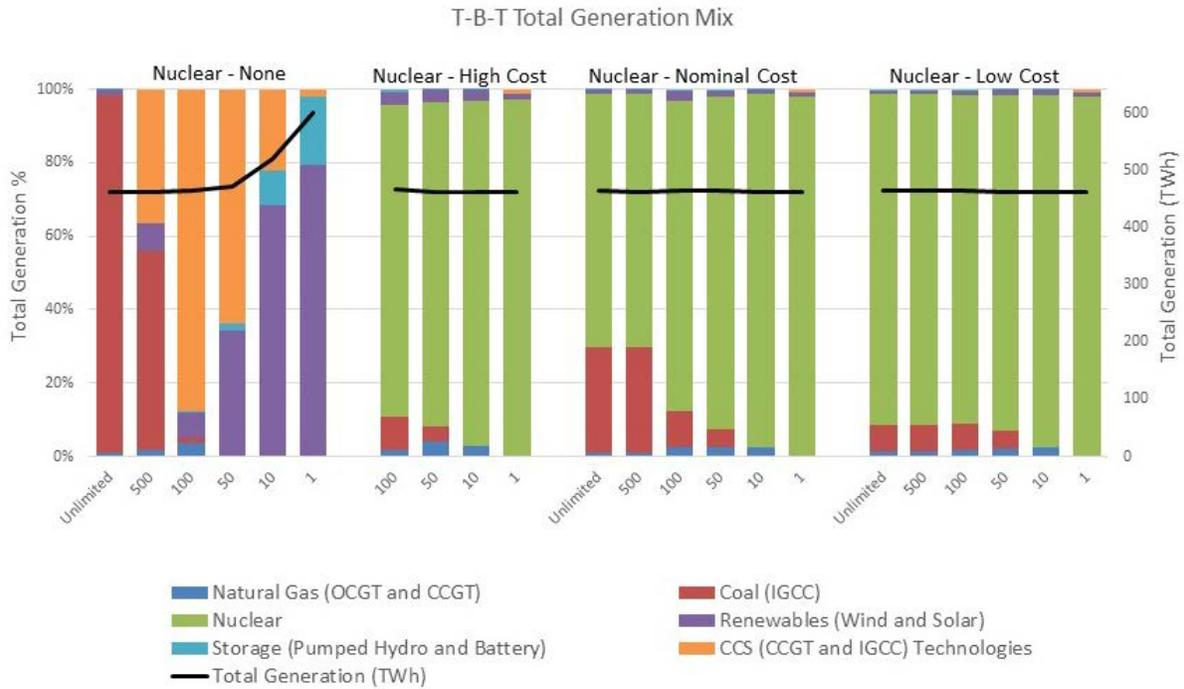
Fig. 5.1.c. TBT Total Generation Mix (left) and Total Generation (right; black line) versus Carbon Dioxide Constraint
