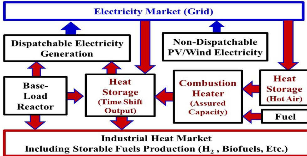
Fig. 9.1. Nuclear Cogeneration System with Heat Storage and Assured Peak Heat and Electricity Output
