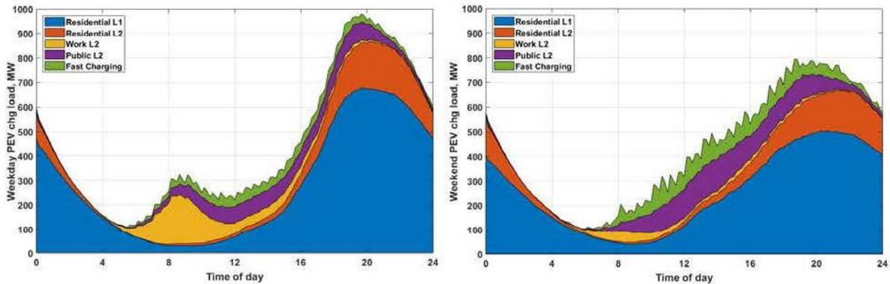
Fig. 7.9. Projected California Electric Vehicle Charging Load in 2025 for Weekdays (left) and Weekends
