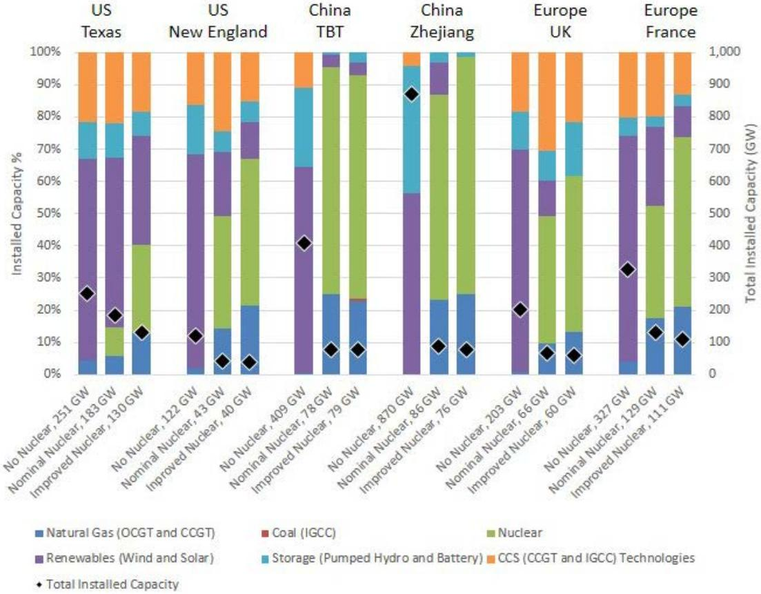
Figure 4.1.d: Generating Capacity for the Six Regions with a Carbon Constraint of 10 g/kWh
