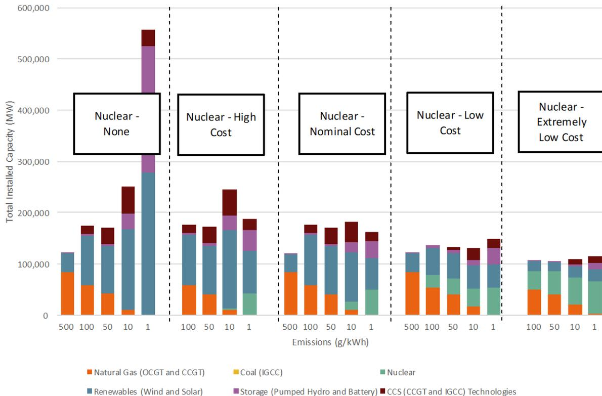
Figure 4.2.a: Optimal Capacity Mixes for Texas
