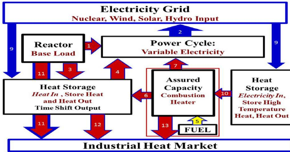
Fig. 7.8. Integrated Nuclear-Renewable Co-generation System
