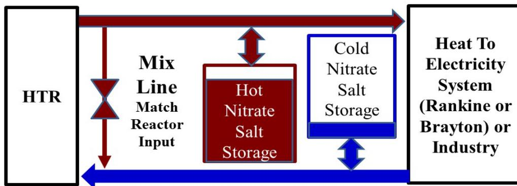
*Fig. D.4. Two-Tank Liquid-Salt Heat Storage*
