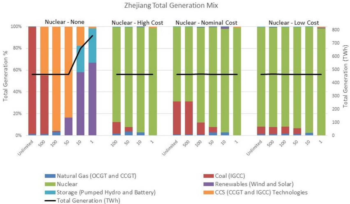
Fig. 5.1.d. Zhejiang Total Generation Mix (left) and Total Generation (right; black line) versus Carbon Dioxide Constraint
