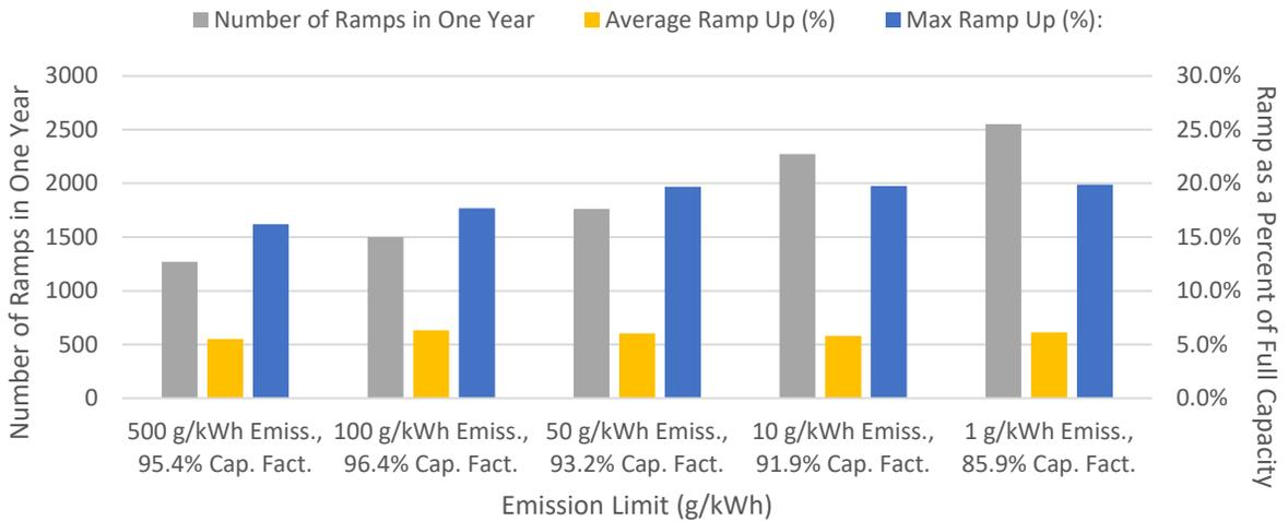
Fig. S.4. T-B-T China Nuclear Operations for Different Carbon Constraints
