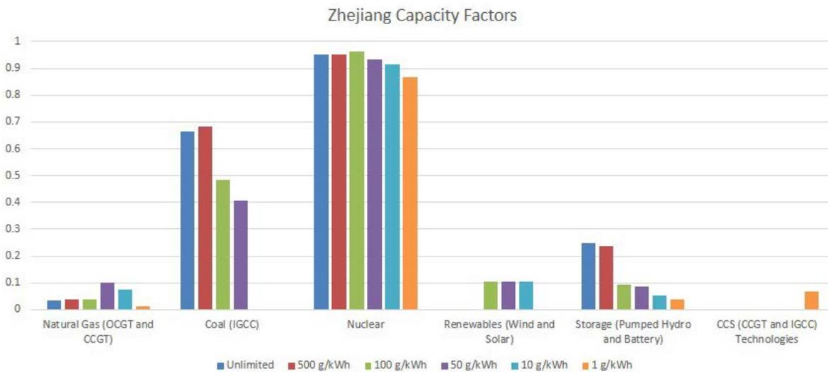
Fig. 6.1.d. Capacity Factors of Generating Technologies in Zhejiang versus CO<sub>2</sub> Emission Limits
