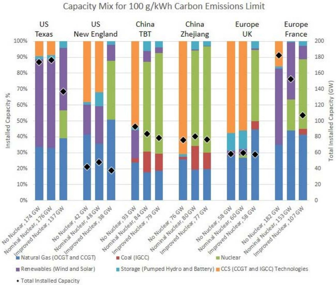
Figure 4.1.b: Generating Capacity for the Six Regions with a Carbon Constraint of 100 g/kWh
