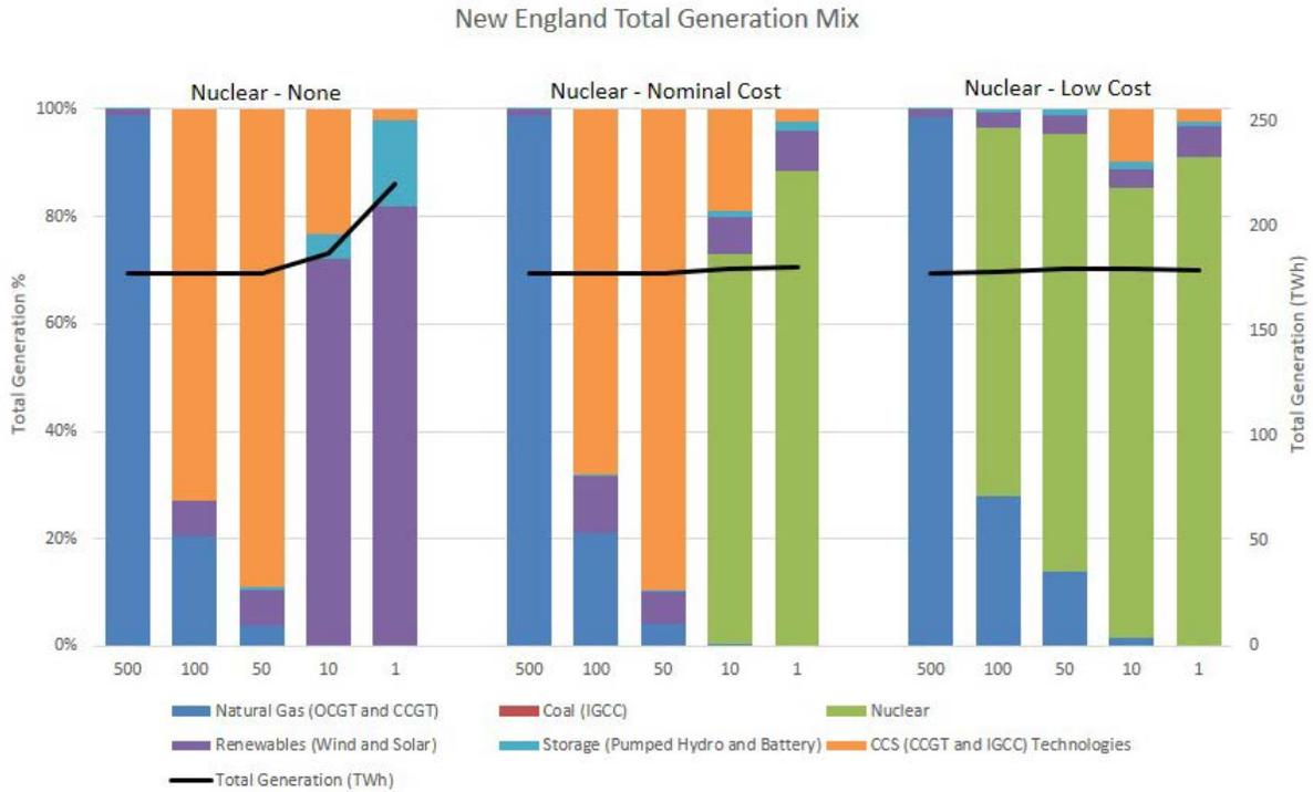
Fig. 5.1.b. New England Total Generation Mix (left) and Total Generation (right, black line) versus Carbon Dioxide Constraint
