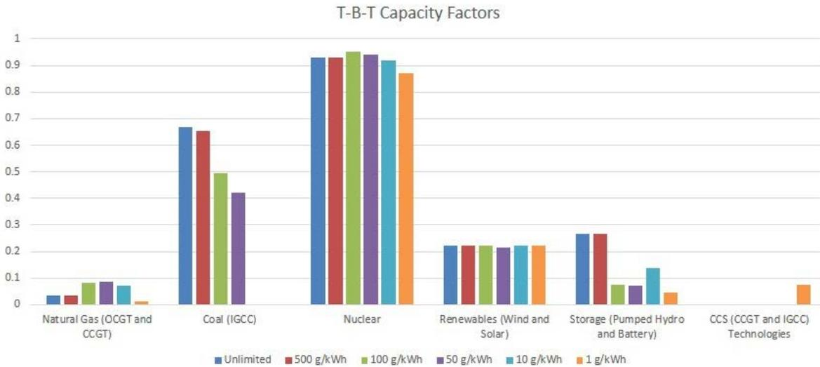
Fig. 6.1.c. Capacity Factors of Generating Technologies in TBT versus CO<sub>2</sub> Emission Limits
