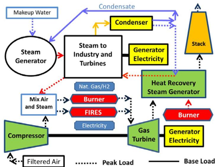
Fig. 8.2. Schematic of Base-load Steam Cycle with Steam-Injection Brayton Topping Cycle
