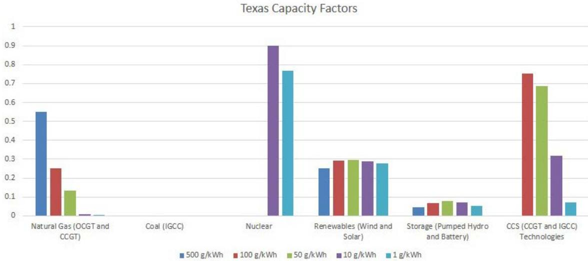
Fig. 6.1.a. Capacity Factors of Generating Technologies in Texas versus CO<sub>2</sub> Emission Limits
