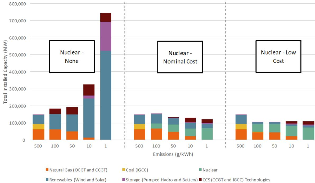
Figure 4.2.f. Optimal Capacity Mix for France
