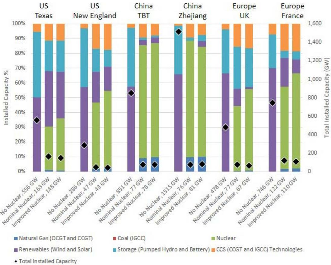
Figure 4.1.e: Generating Capacity for the Six Regions with a Carbon Constraint of 1 g/kWh
