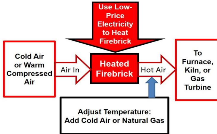
Fig. 7.7 Firebrick Resistance Heated Energy Storage (FIRES)
