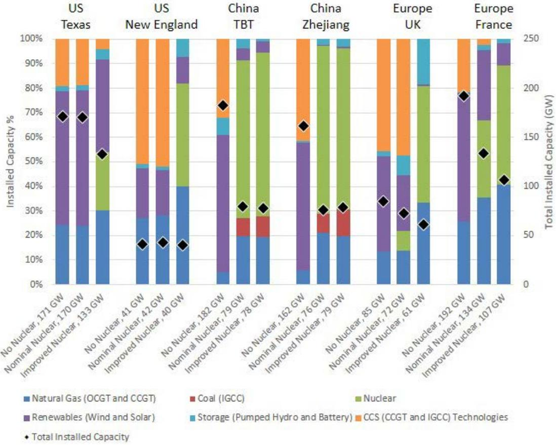
Figure 4.1.c: Generating Capacity for the Six Regions with a Carbon Constraint of 50 g/kWh
