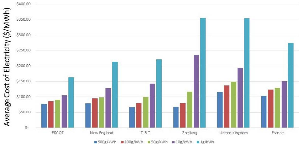
Fig. 3.3. Average Cost of Electricity for Non-Nuclear Scenarios versus Carbon Constraint
