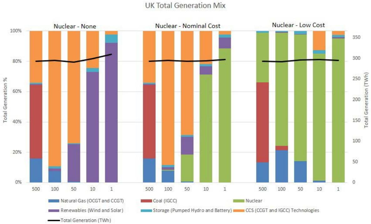
Fig. 5.1.e. United Kingdom Total Generation Mix (left) and Total Generation (right; black line) versus Carbon Dioxide Constraint
