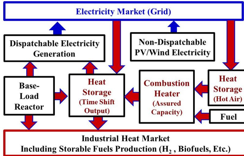
Fig. 7.1 Low-Carbon System Design
