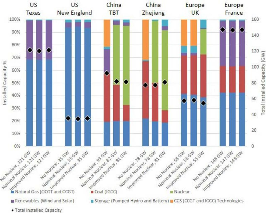
Figure 4.1.a: Generating Capacity for the Six Regions with a Carbon Constraint of 500 g/kWh
