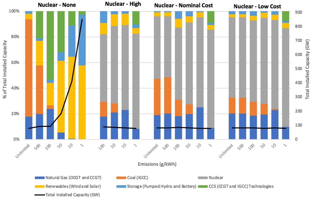
Fig. 4.3.a. Optimal Capacity Mix for T-B-T over a Wide Range of Nuclear Plant Costs
