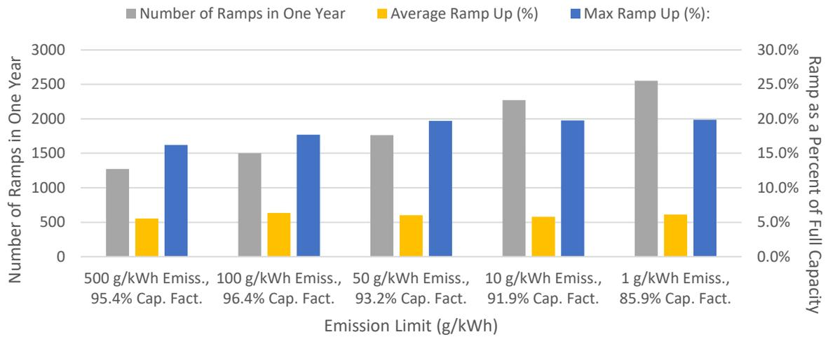
Fig. 6.3.c T-B-T Nuclear Power Ramping
