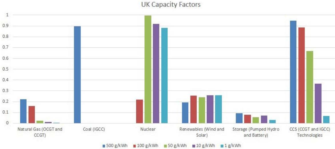
Fig. 6.1.e. Capacity Factors of Generating Technologies in the United Kingdom vs. CO<sub>2</sub> Emission Limits
