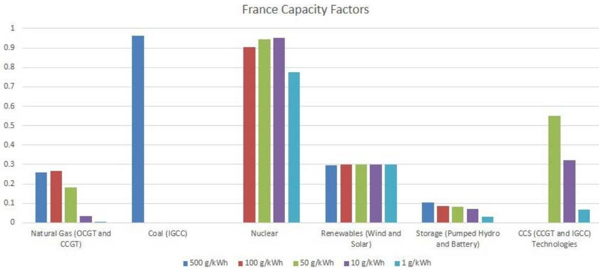
Fig. 6.1.f. Capacity Factors of Generating Technologies in France vs. CO<sub>2</sub> Emission Limits
