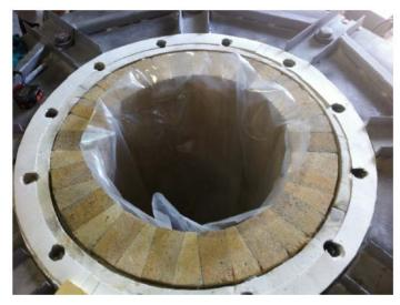
Refractory-lined, stainless-steel tank tested for use with chloride salts (Jonemann 2013).
