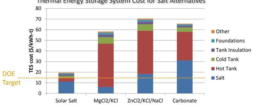
Thermal Energy Storage System Cost for Salt Alternatives
