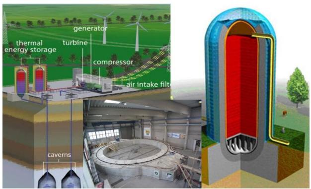
Project Adele system, laboratory section of prestress pressure vessel and schematic of the pressure vessel. Courtesy of General Electric, RWE AG, and Zublin
