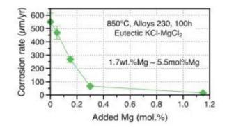
If salt chemistry  $-O_2$ ,  $H_2O$ content - can be controlled, corrosion can be managed
