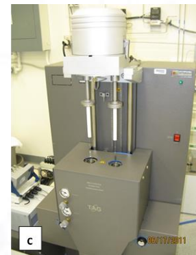
Temperature control and continuous weight measurement
