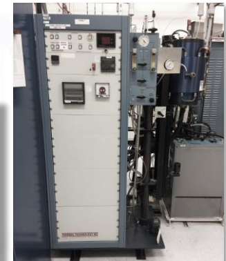
High temperature vacuum furnace 1 h @ 1800 °C
