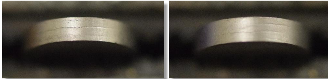
Examples of surface fissures prompting rejection
