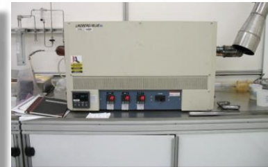
Carbonization furnace 0.5 h @ 900 °C
