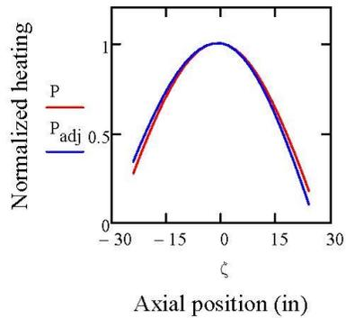
Note: The unsymmetric heating profile (blue trace) was shown to improve temperature calculations in the AGC tests as compared to using the symmetric heating profile (red trace); see ECAR-2562 and ECAR-2322.
