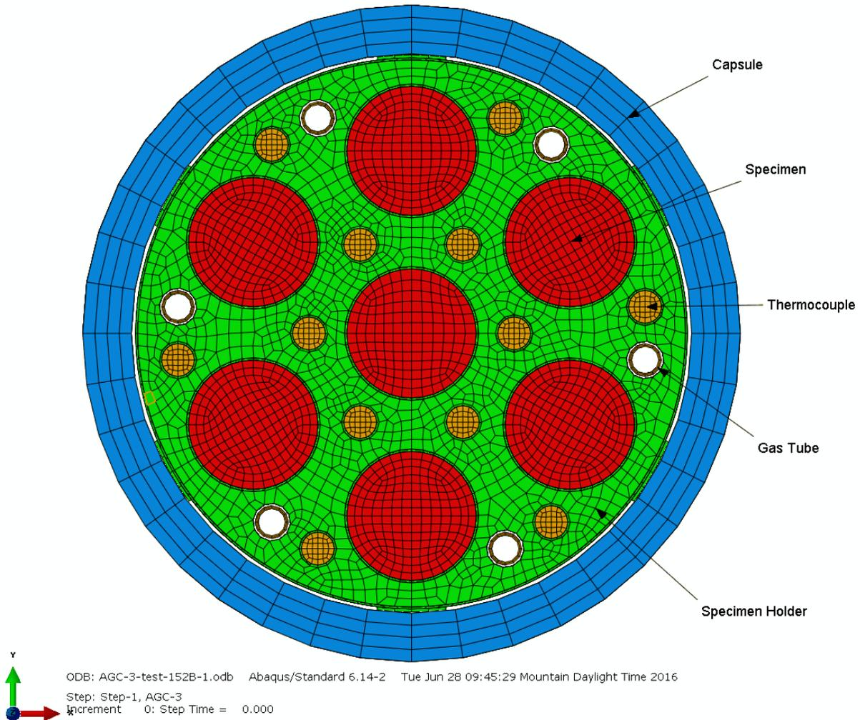
Figure 3. Model geometry and finite element mesh (cross-sectional view of the experiment).
