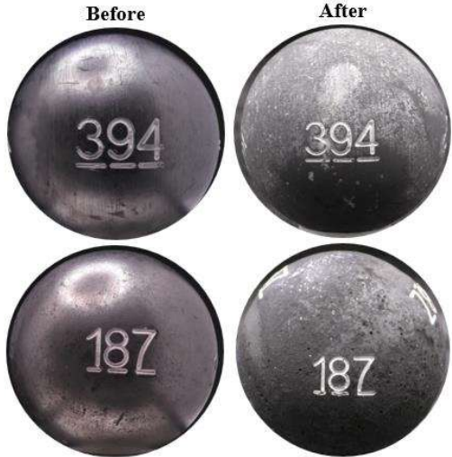
Comparative visuals of pebbles pre- and post-abrasion test with thermal exposure, captured via Panasonic camera
