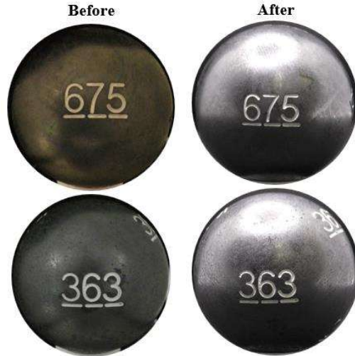
Comparative visuals of pebbles pre- and post-abrasion test without thermal exposure, captured via Panasonic camera
