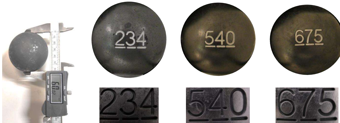
6.0 cm Graphite pebbles carved using Model Mazak VTC-20B and tagged with ceramic patterns
