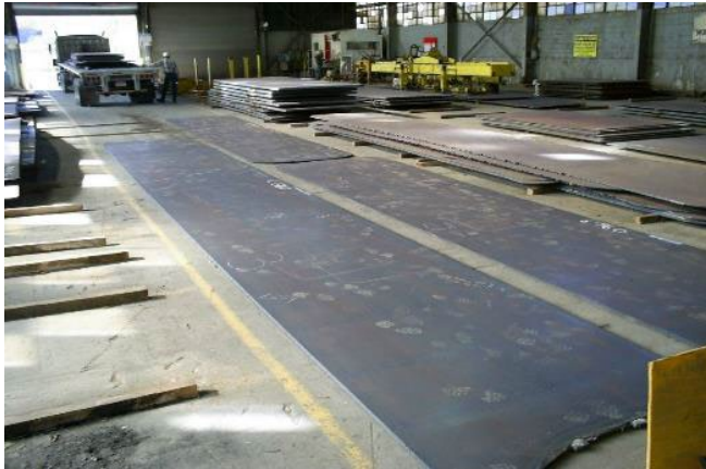
Photograph of first commercial heat A709 plates in as-rolled condition at vendor location
