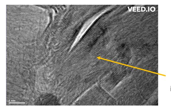
Crack closure under irradiation
