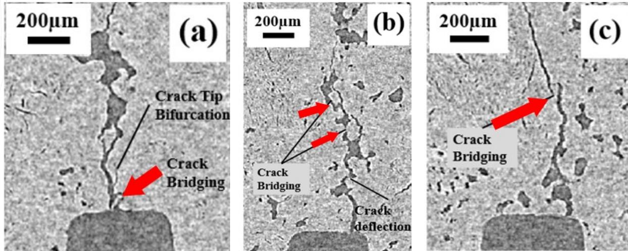
Crack bridging by uncracked ligament: (a) in the filler, (b) in the binder, (c) at the filler-binder boundary
