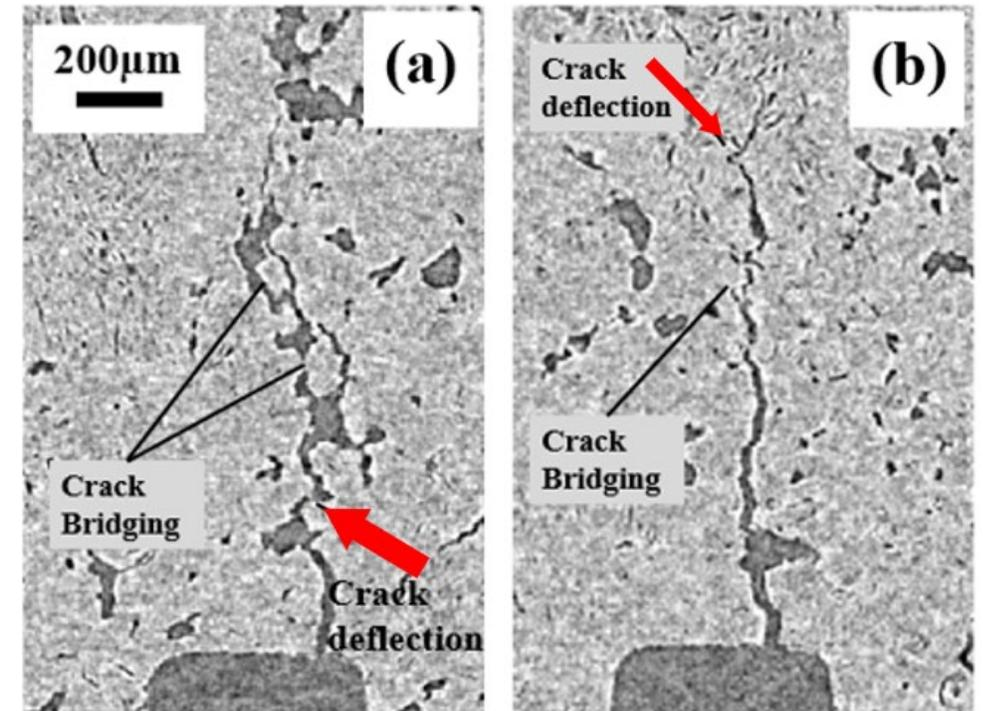
Crack deflection due to thermal crack and gas entrapment pores
