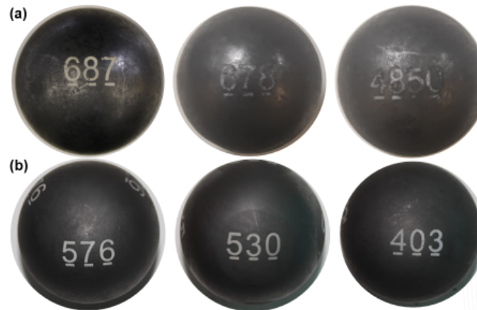
Ceramic Patterns on graphite pebbles (a) Without treatment (b) With treatment
