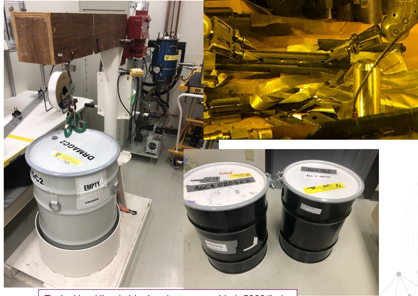
Typical lead lined shipping drum assembly (~5000 lbs) and new small quantity shipping drums (~50 lbs)
